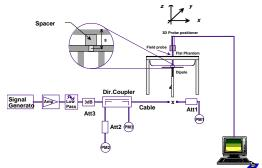
Figure 7.1 Dipole Validation Test Setup
