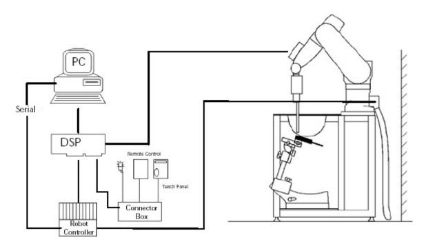
Figure 2.1 SAR Measurement System Setup
