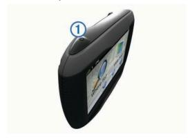
**NOTE:** If you hold the Power key for less than 5 seconds, the device enters sleep mode (page 3).
