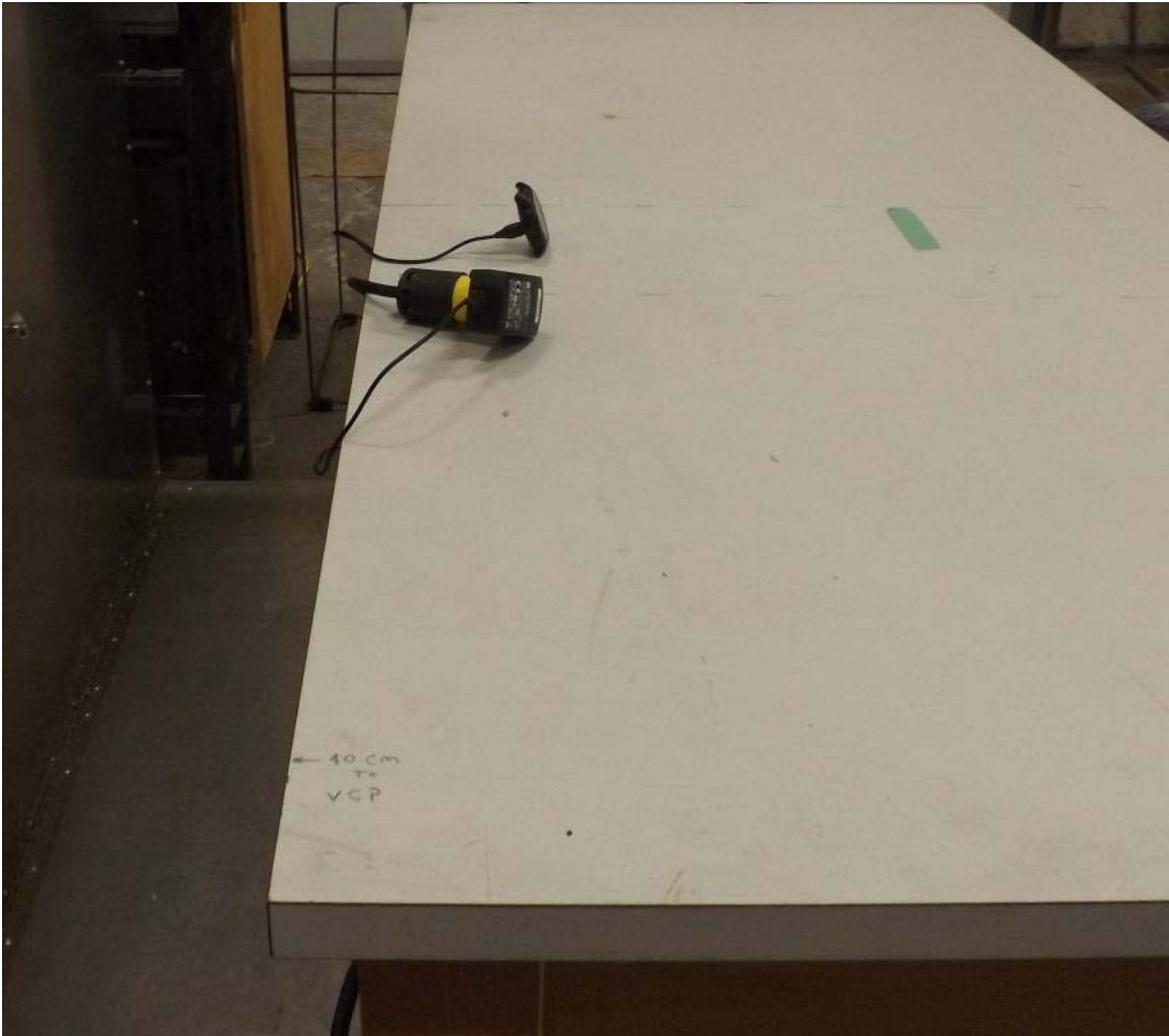
Figure E16.10 – Setup, Line Conducted Measurements
