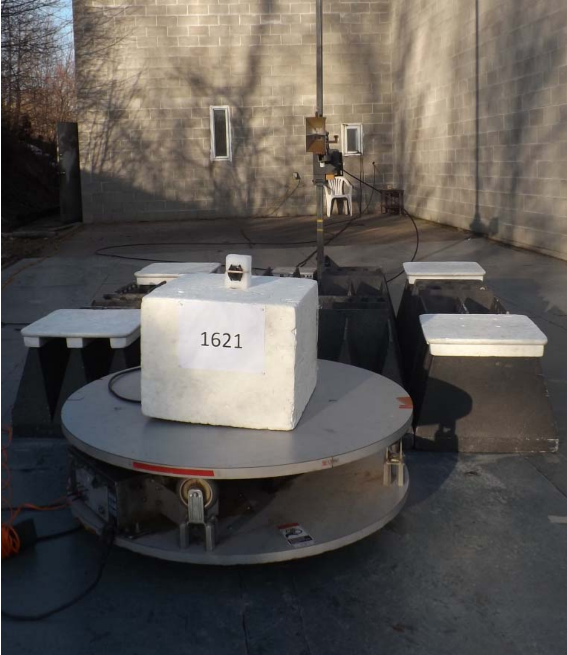
Figure E16.6 – Setup, Radiated Rx Measurements, 1 - 18GHz
