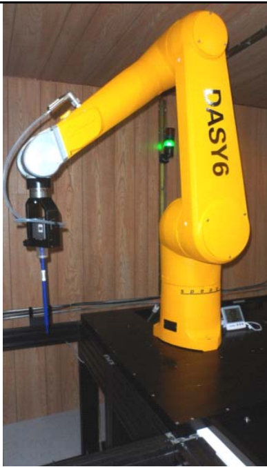
DASY 6 SAR System with SAM Phantom
