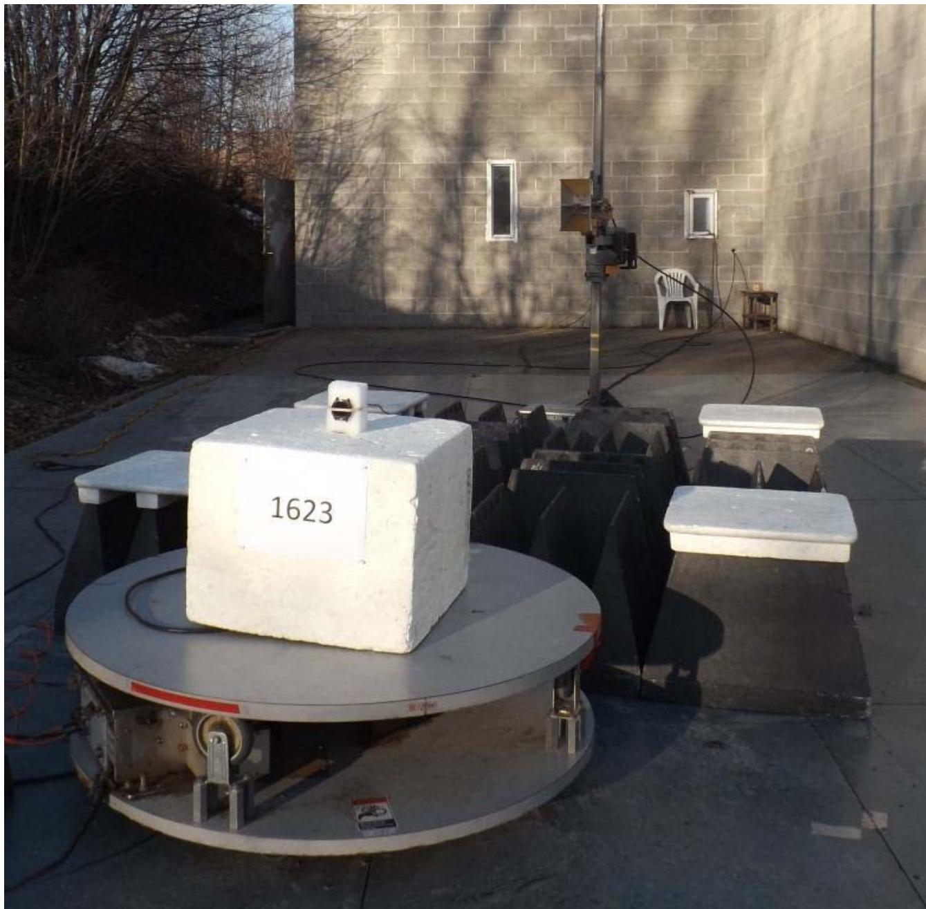
Figure E16.6 – Setup, Radiated Rx Measurements, 1 - 18GHz
