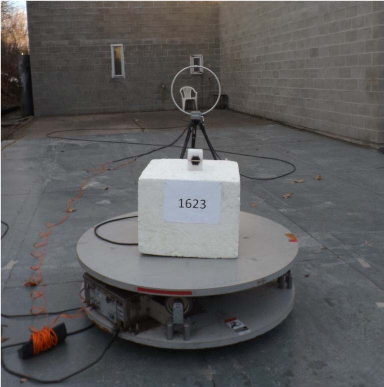
Figure E16.2 – Setup, Radiated Measurements <30MHz
