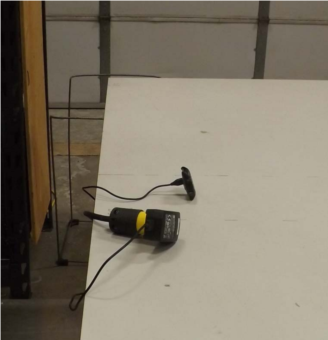
Figure E16.10 – Setup, Line Conducted Measurements
