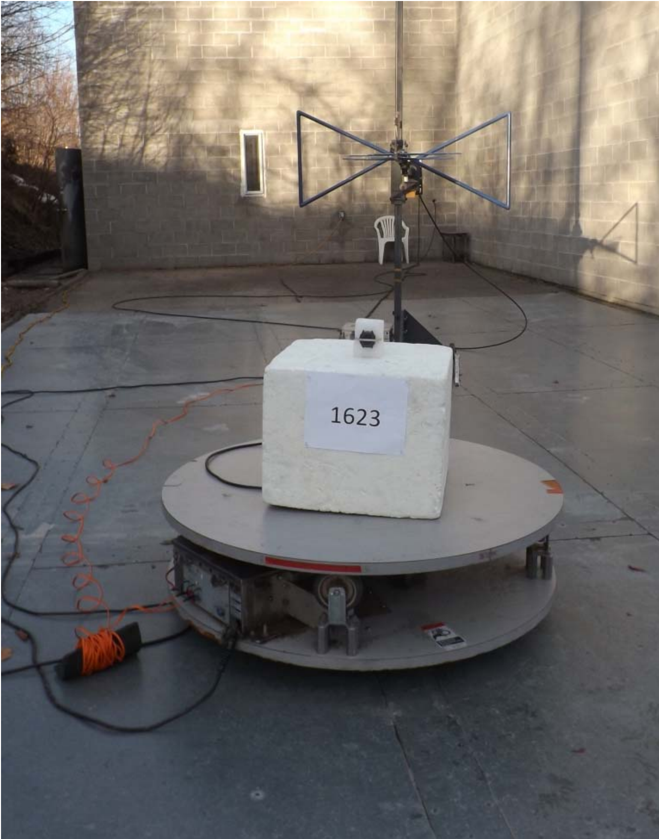
Figure E16.3 – Setup, Radiated Measurements 30 – 1000MHz
