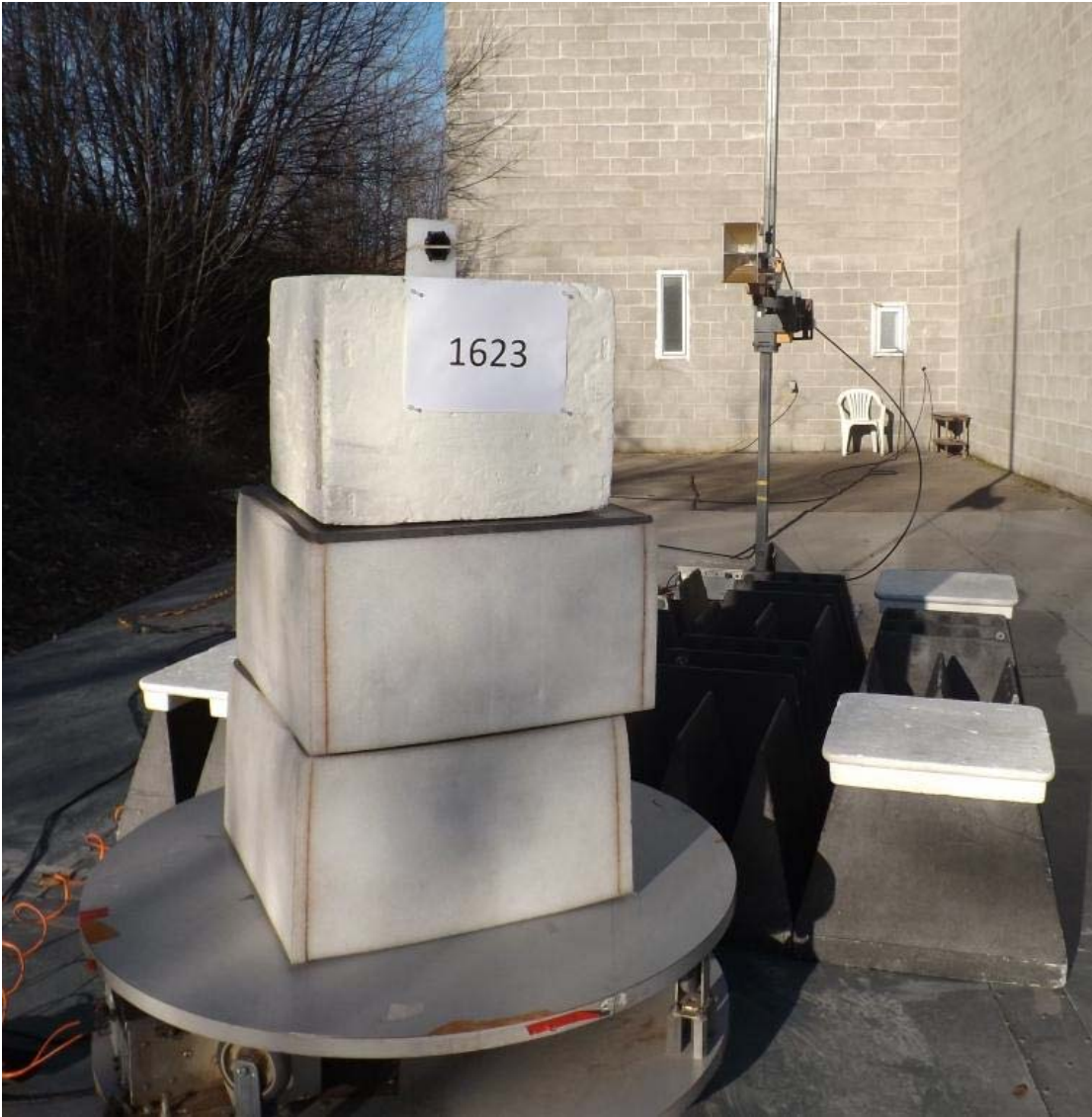
Figure E16.4 – Setup, Radiated Measurements, 1 – 18GHz
