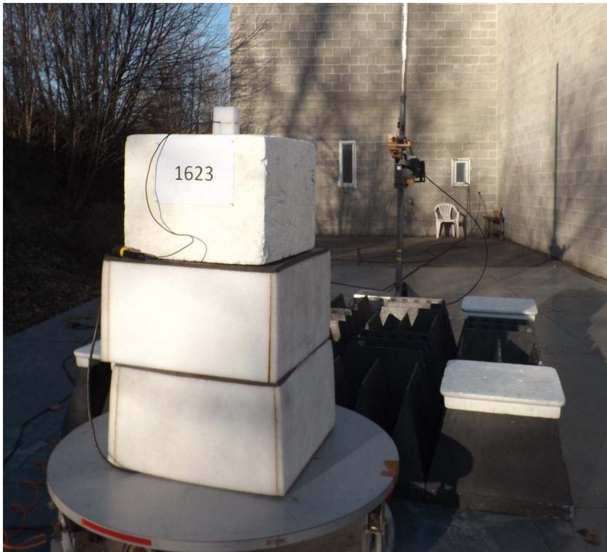
Figure E16.5 – Setup, Radiated Measurements, 18 - 26GHz
