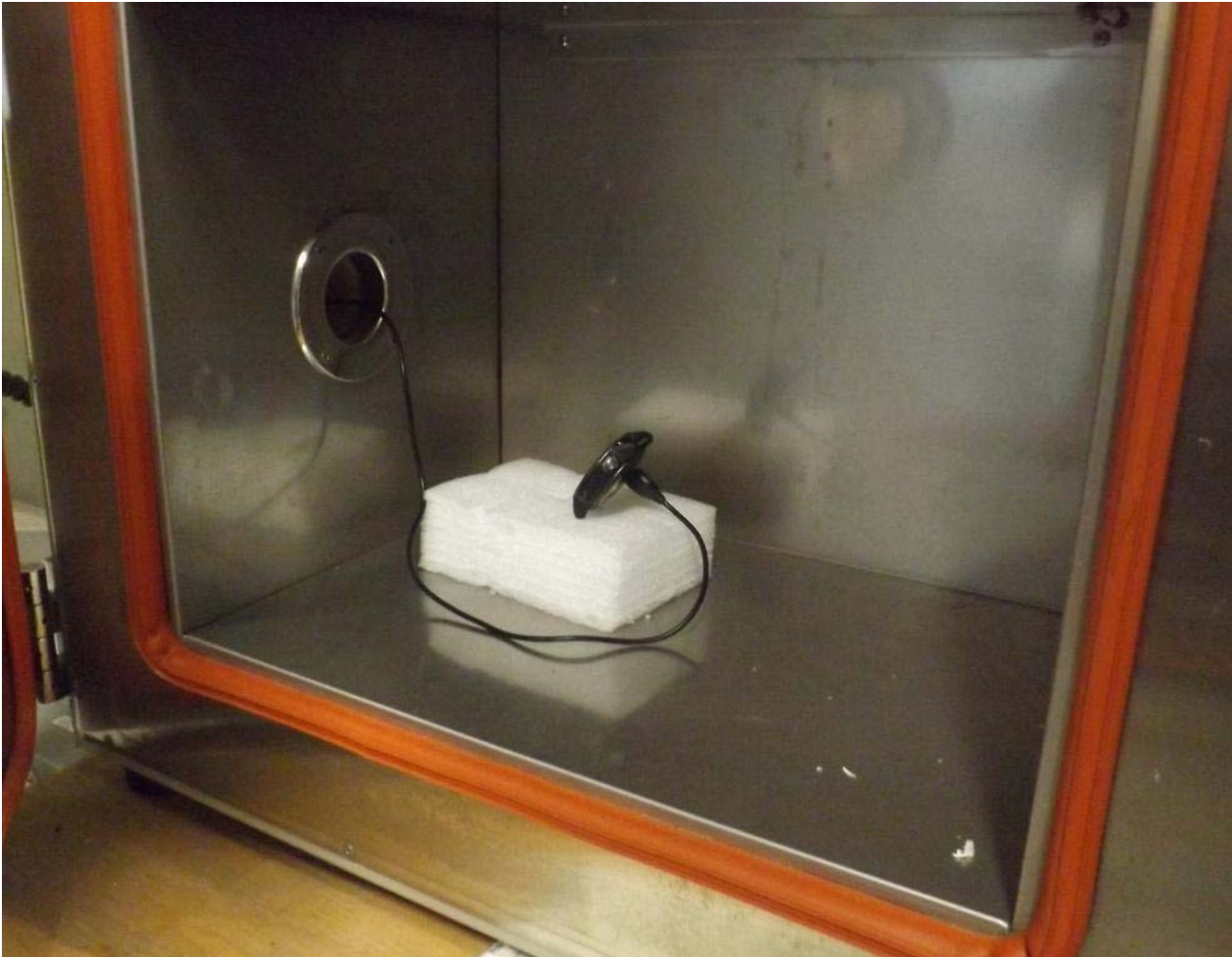
Figure E16.8 – Setup, NFC Frequency Stability Measurements
