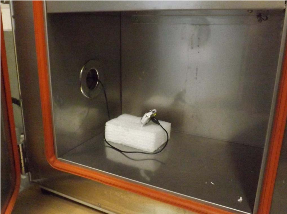
Figure E16.8 – Setup, NFC Frequency Stability Measurements
