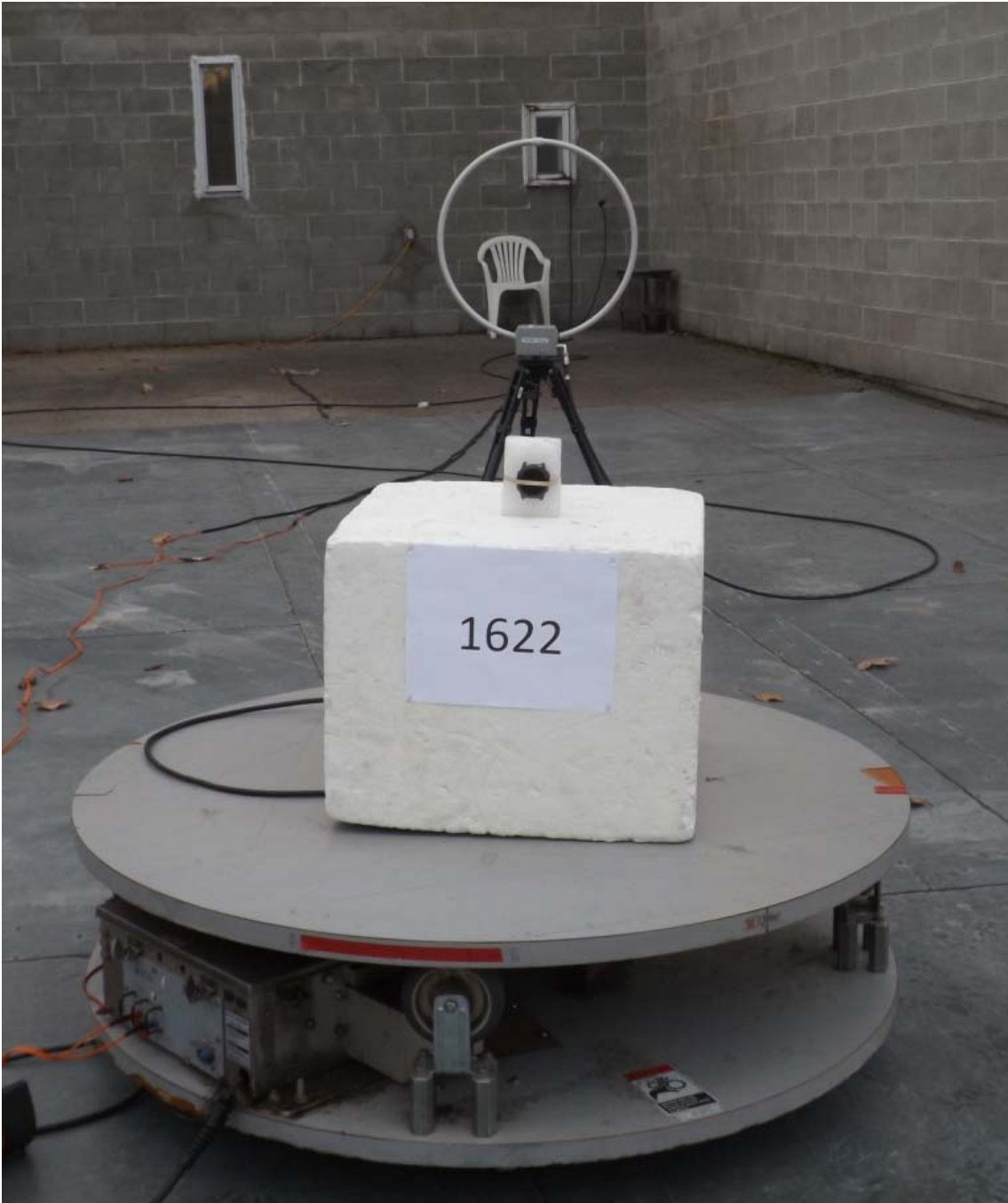
Figure E16.2 – Setup, Radiated Measurements <30MHz
