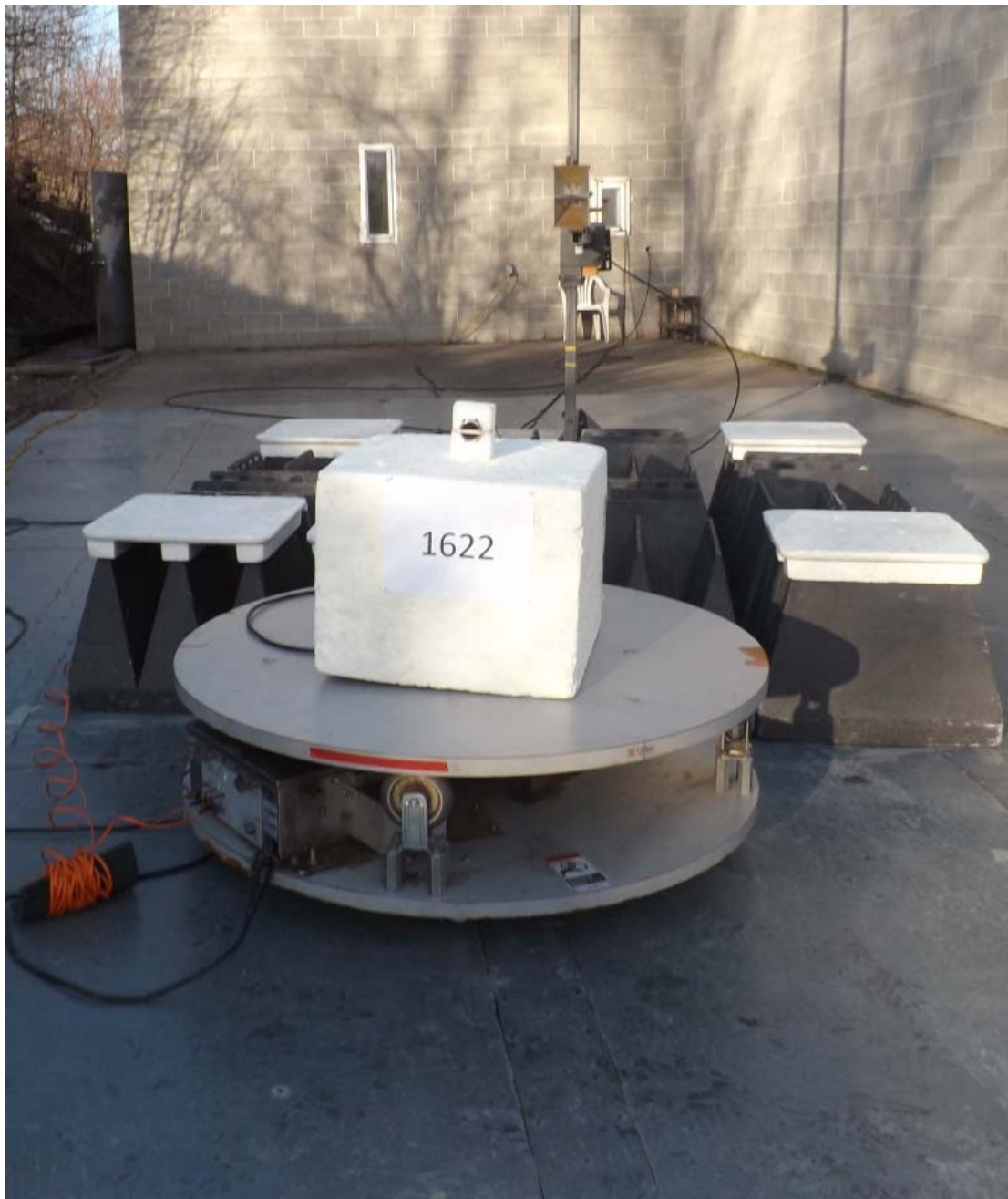
Figure E16.6 – Setup, Radiated Rx Measurements, 1 - 18GHz
