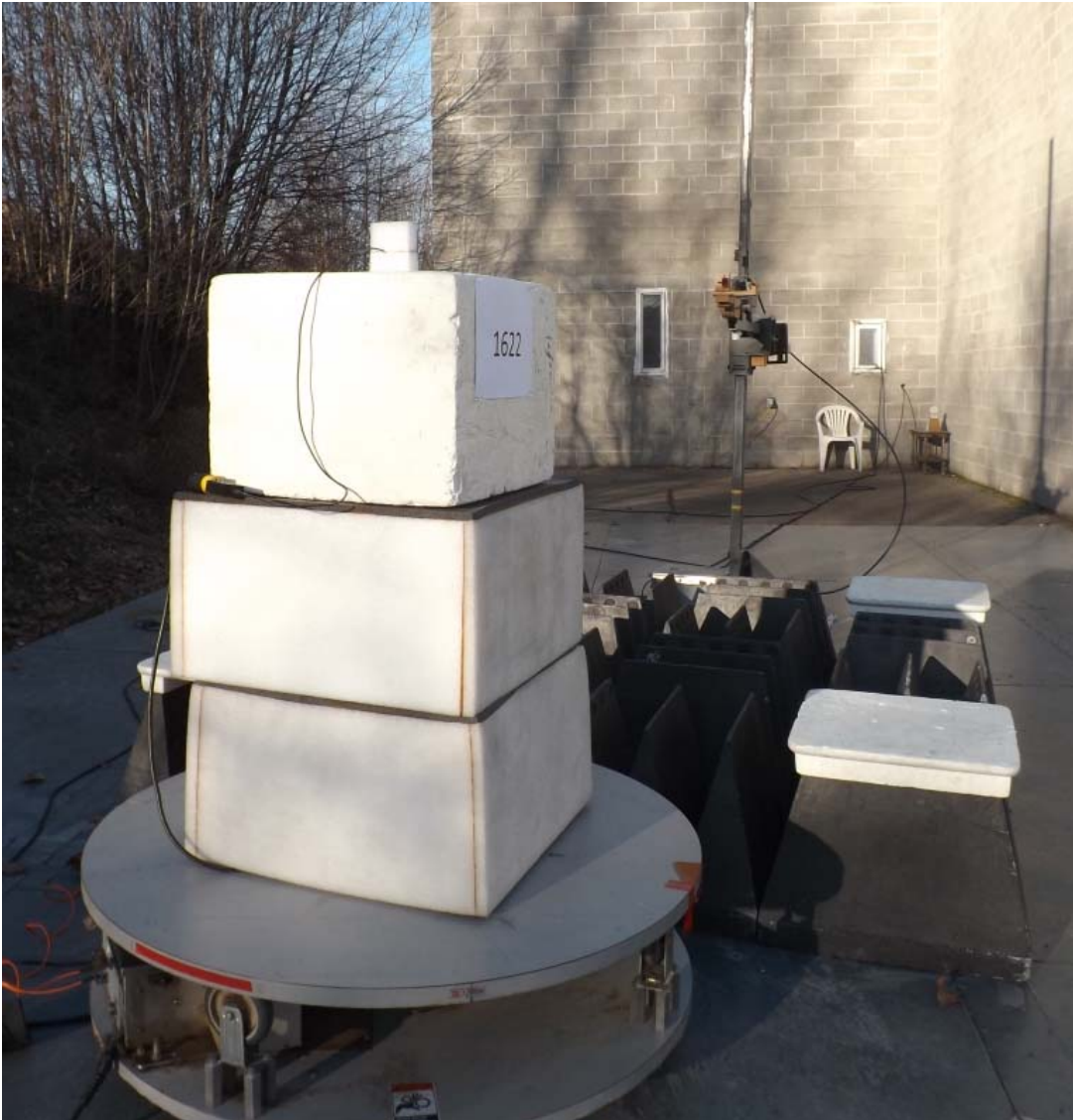
Figure E16.5 – Setup, Radiated Measurements, 18 - 26GHz
