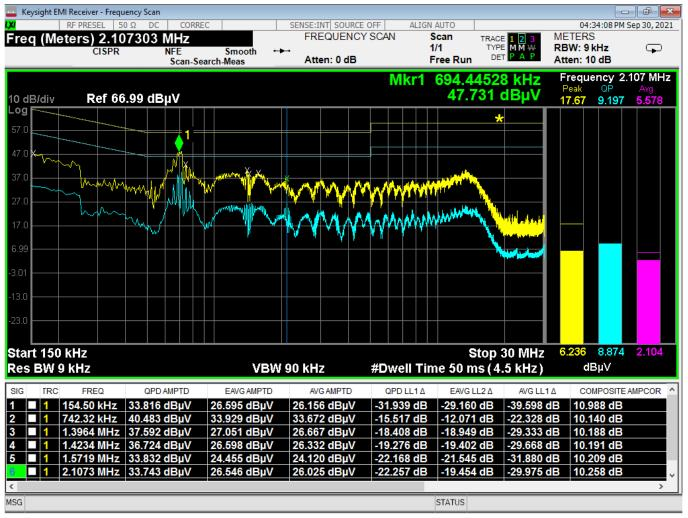
Figure 17 - Conducted Emissions Plot, Line, TX
