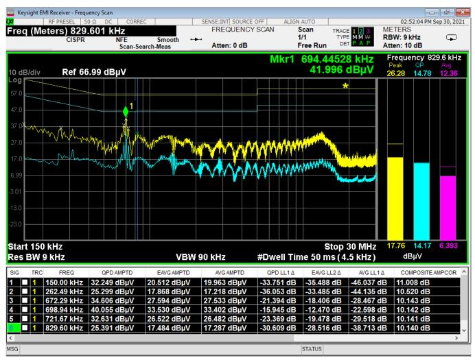
Figure 20 - Conducted Emissions Plot, Neutral, IDLE
