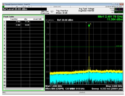
Figure 8 - Radiated Emissions Plot, BTBR, 1G - 3.6G
