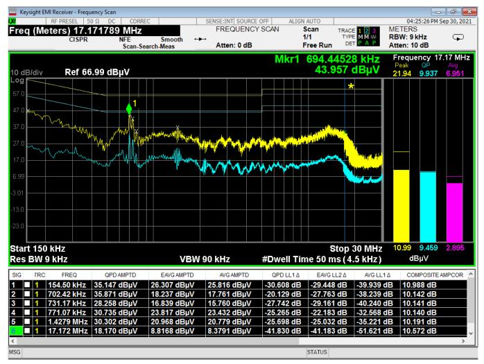
Figure 11 - Conducted Emissions Plot, Neutral, TX
