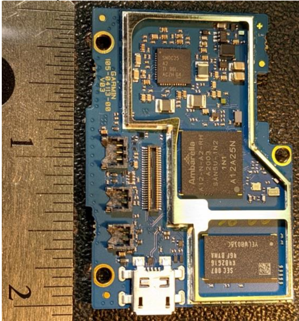
Main Board top side shield removed
