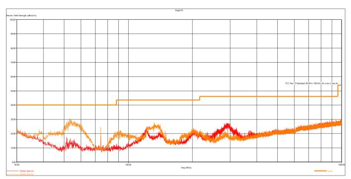
Figure 8 - Radiated Emissions Plot, BT EDR 3MB
