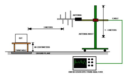
Figure 2 - Radiated Emissions Test Setup
