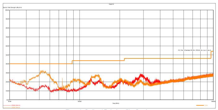
Figure 6 - Radiated Emissions Plot, Receive
