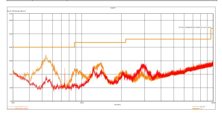
Figure 8 - Radiated Emissions Plot, 802.11b, High Data Rate, Low Ch
