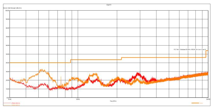
Figure 4 - Radiated Emissions Plot, Receive
