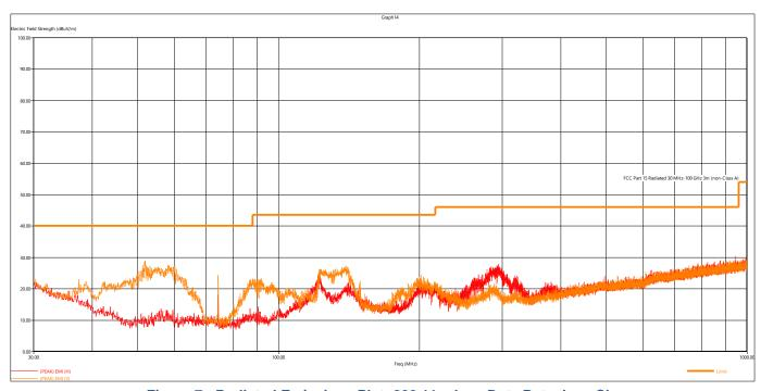
Figure 7 - Radiated Emissions Plot, 802.11n, Low Data Rate, Low Ch
