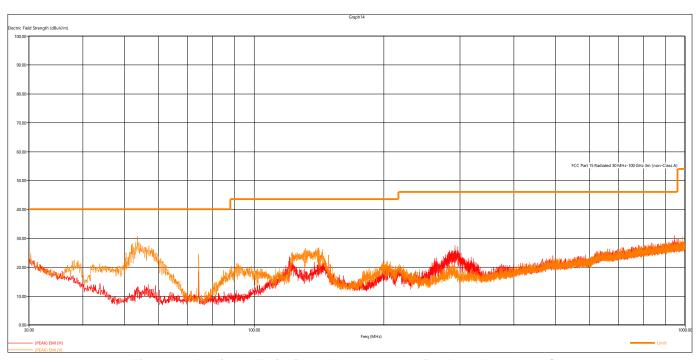
Figure 9 - Radiated Emissions Plot, 802.11g, High Data Rate, Low Ch
