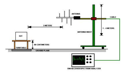
Figure 3 - Radiated Emissions Test Setup
