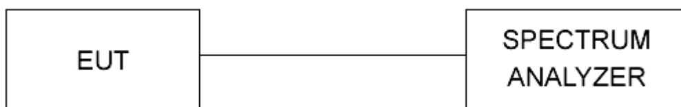
Figure 1 - Bandwidth Measurements Test Setup
