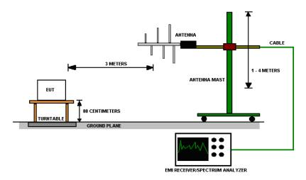
Figure 2 - Radiated Emissions Test Setup
