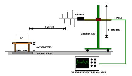
Figure 4 - Radiated Emissions Test Setup
