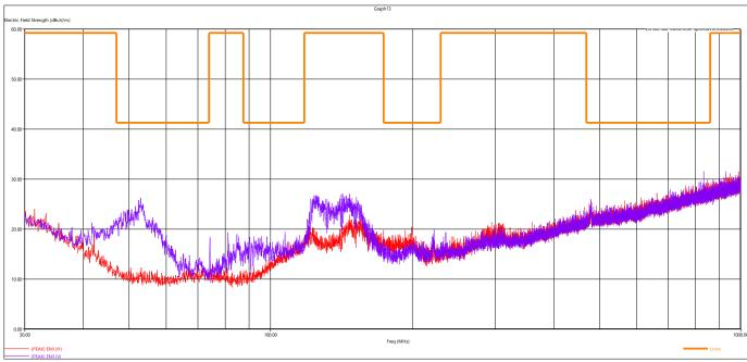
Figure 7 - Radiated Emissions Plot, BT EDR 2MB
