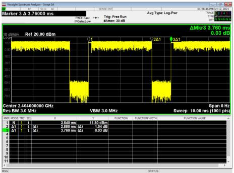
Figure 3 – 2EDR Duty Cycle DCCF (Duty Cycle Correction Factor) = 20 \* Log(Duty Cycle / 100) -2.27 = 20 \* Log(77 / 100)
