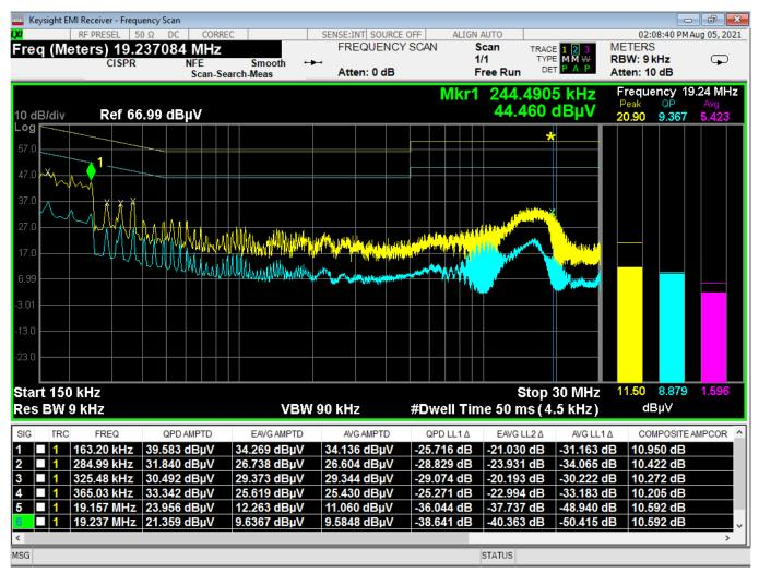
Figure 17 - Conducted Emissions Plot, Line, IDLE
