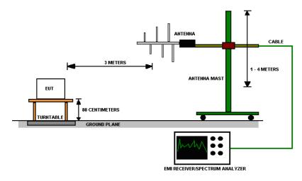
Figure 2 - Radiated Emissions Test Setup
