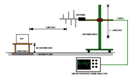
Figure 5 - Radiated Emissions Test Setup
