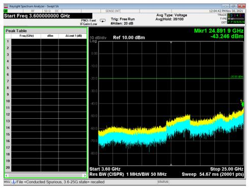
Figure 14 - Radiated Emissions Plot, 3EDR, 3.6G – 25G
