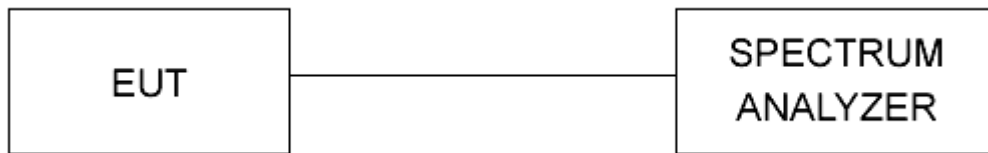
Figure 1 - Bandwidth Measurements Test Setup
