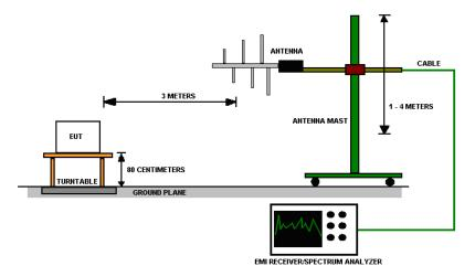
Figure 4 - Radiated Emissions Test Setup
