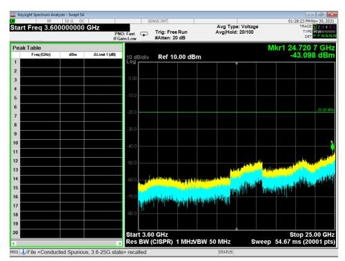
Figure 9 - Radiated Emissions Plot, BTBR, 3.6G - 25G
