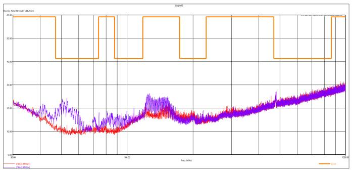
Figure 5 - Radiated Emissions Plot, Receive
