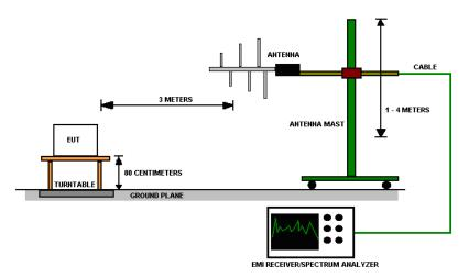
Figure 2 - Radiated Emissions Test Setup
