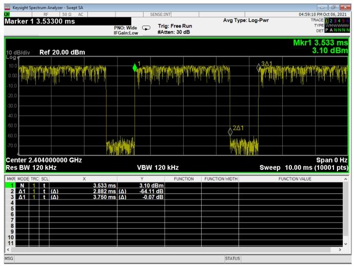
Figure 3 - Radiated Emissions Plot, BTBR, Duty Cycle
