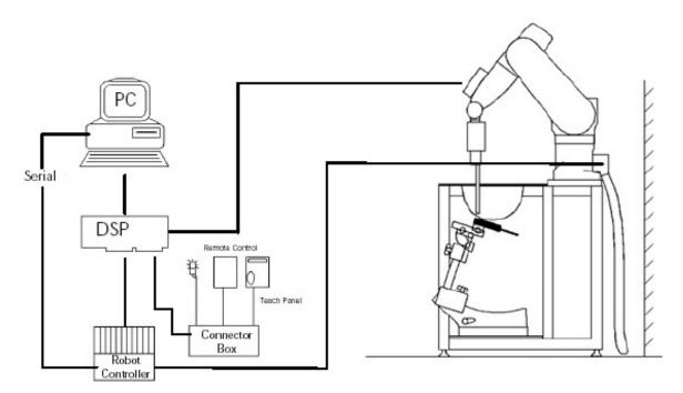
Figure 2.1 SAR Measurement System Setup
