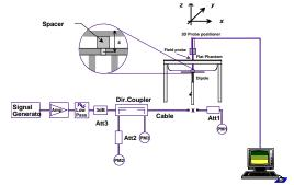
Figure 7.1 Dipole Validation Test Setup
