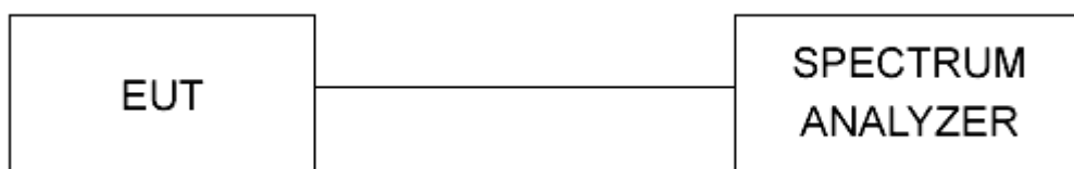
Figure 1 - Bandwidth Measurements Test Setup
