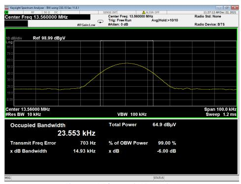
Figure 6 - NFC Occupied Bandwidth
