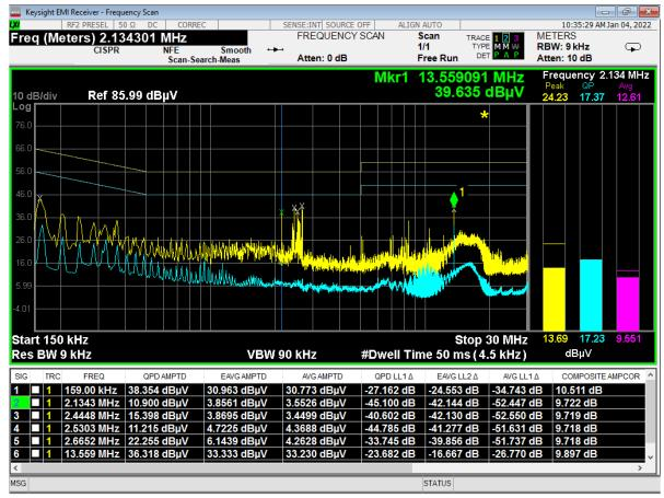
Figure 8 - Conducted Emissions Plot, Neutral, NFC
