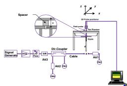
Figure 7.1 Dipole Validation Test Setup
