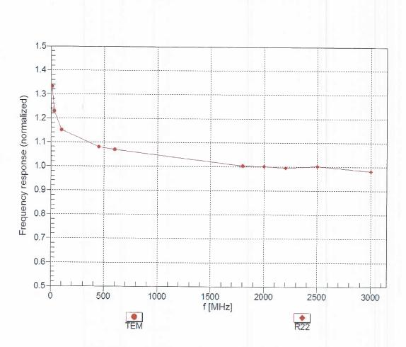
Frequency Response of E-Field (TEM-Cell:ifi110 EXX, Waveguide: R22)
