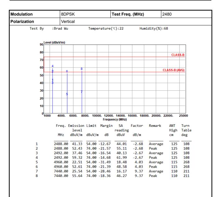
Note 1: Emission Level (dBuV/m) = SA Reading (dBuV) + Factor\* (dB/m)
