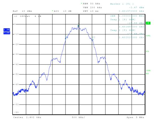
Figure 3 Plot of Transmitter Emissions (99% Occupied Bandwidth)
