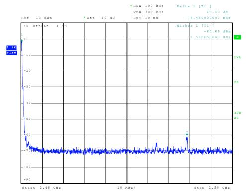
Figure 5 Plot of Transmitter Emissions (High Band Edge)
