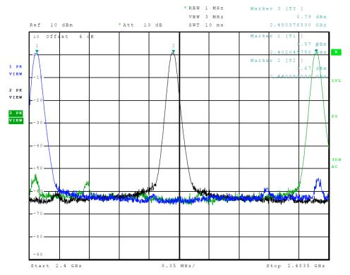
Figure 1 Plot of Transmitter Emissions (Operation in 2402-2480 MHz)
