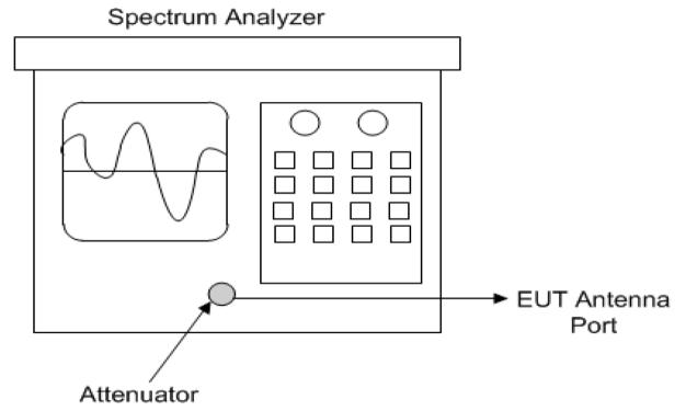
Diagram 1 Test arrangement for Antenna Port Conducted emissions
