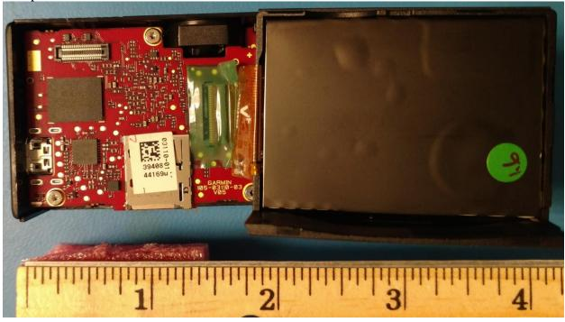
Sensor Board with antenna identification
