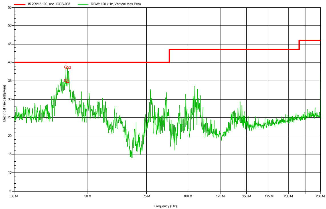
Plot 1a: radiated emissions of the EUT, Antenna vertical, in the range 30 – 250 MHz (pre-scan peak values shown)
