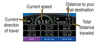
Touch **Reset Trip** to reset all information on the Trip Computer. To reset the Maximum Speed, touch **Reset Max**.
