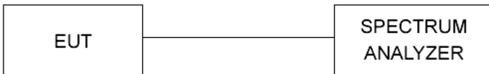
Figure 1 - Bandwidth Measurements Test Setup
