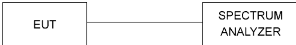
Figure 1 - Bandwidth Measurements Test Setup
