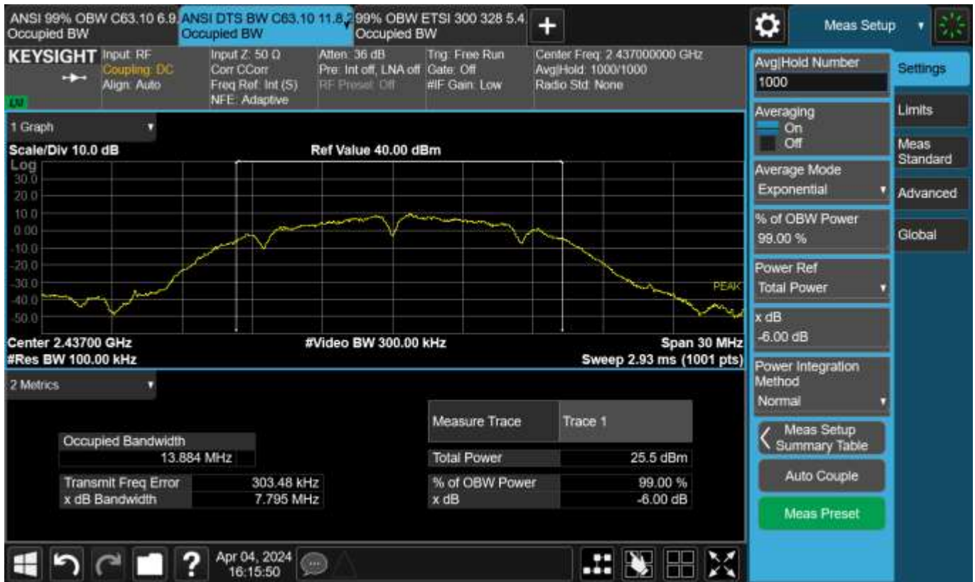
Figure TR06.4: Bandwidth data for 802.11b 2 Mbps at channel 6
