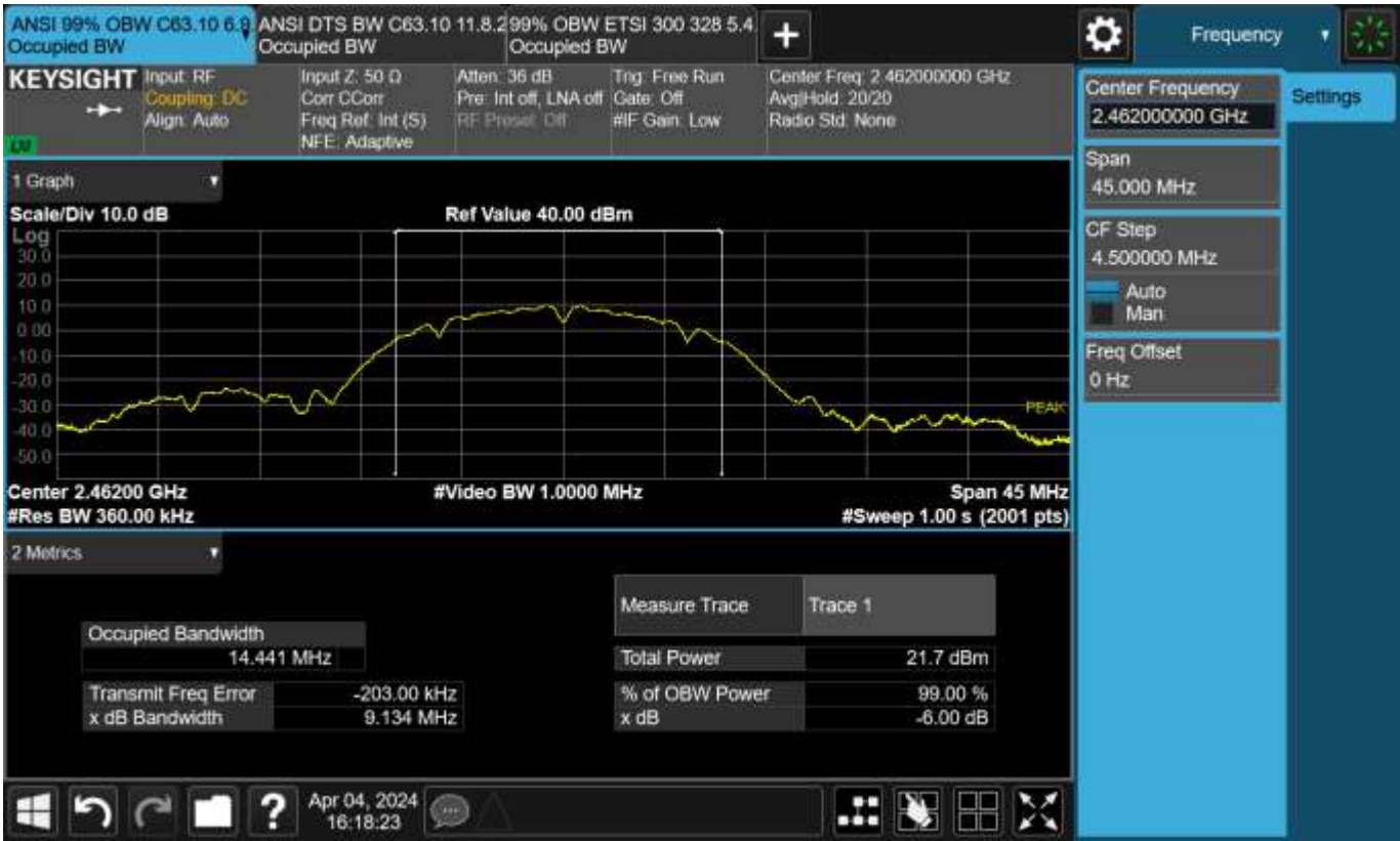
Figure TR10.4: Occupied bandwidth data for 802.11b 2 Mbps at channel 11
