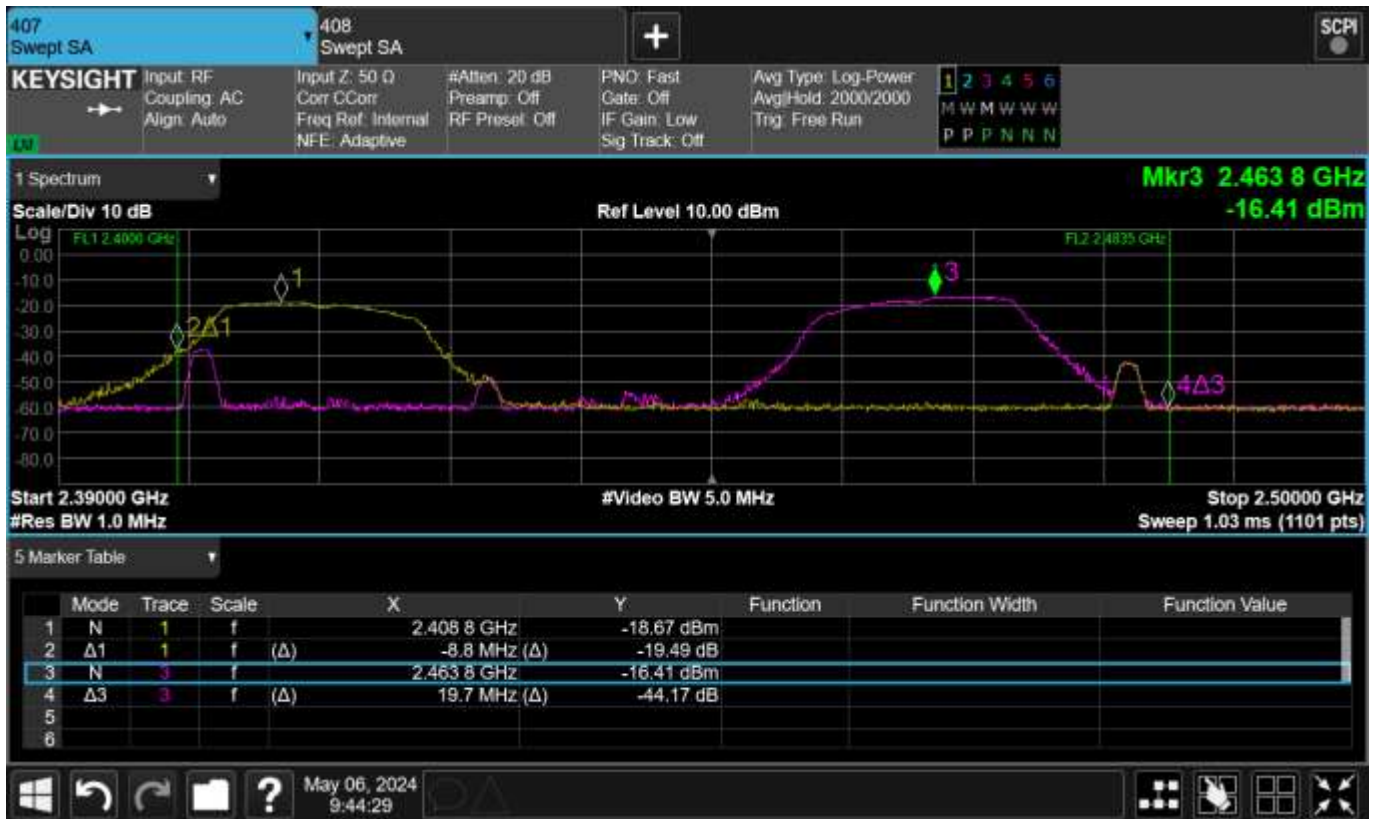
Figure TR44.3: Spectral plot for 20 °C and 5.75 V test condition
