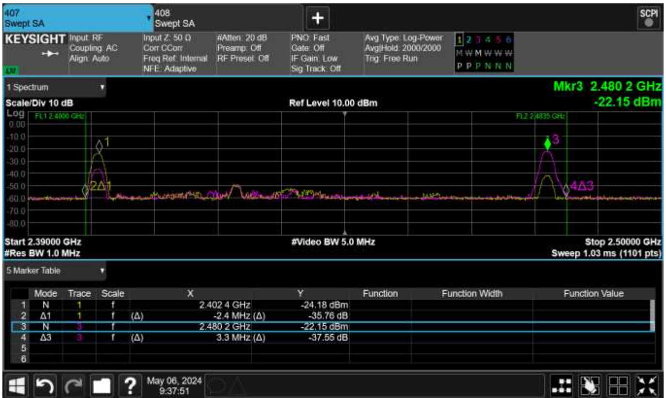
Figure TR43.3: Spectral plot for 20 °C and 5.75 V test condition
