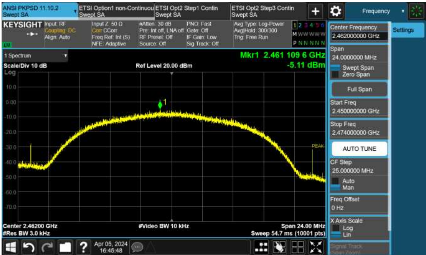
Figure TR19.4: Test data for 802.11 b 5.5 Mbps channel 11
