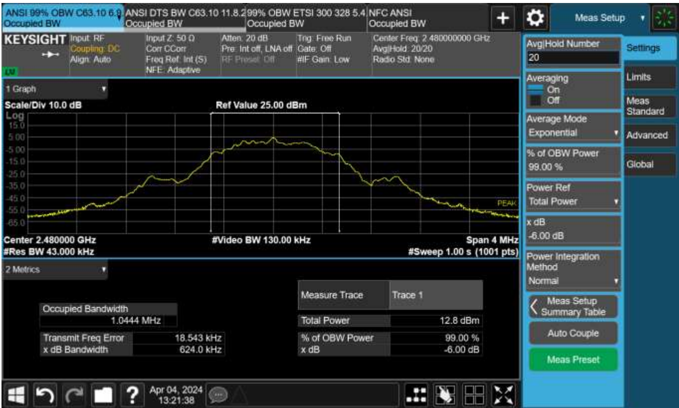
Figure TR10.2: Occupied bandwidth data for BLE at high channel (2480 MHz)
