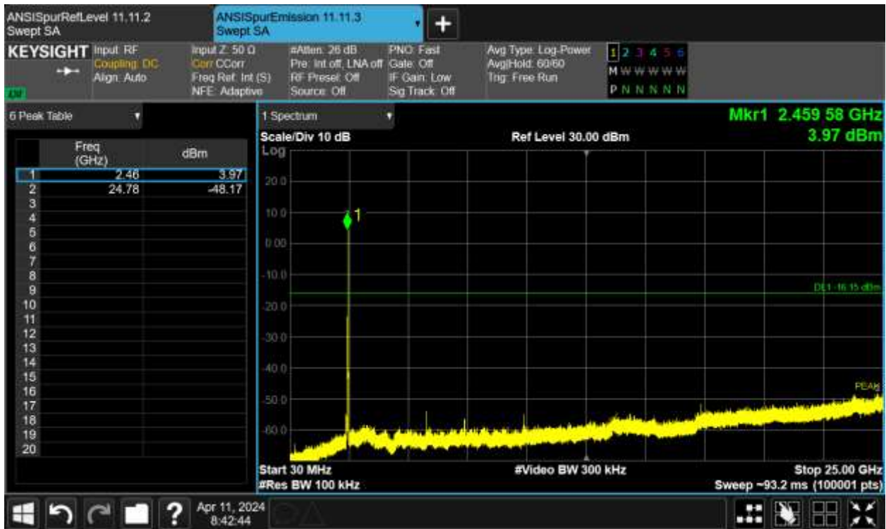
Figure TR27.9 Spectral data for IEEE 802.11 G 9 Mbps on Ch.11
