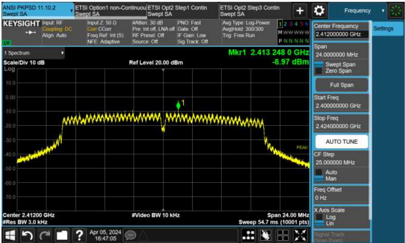
Figure TR19.5: Test data for 802.11 g 9 Mbps channel 1
