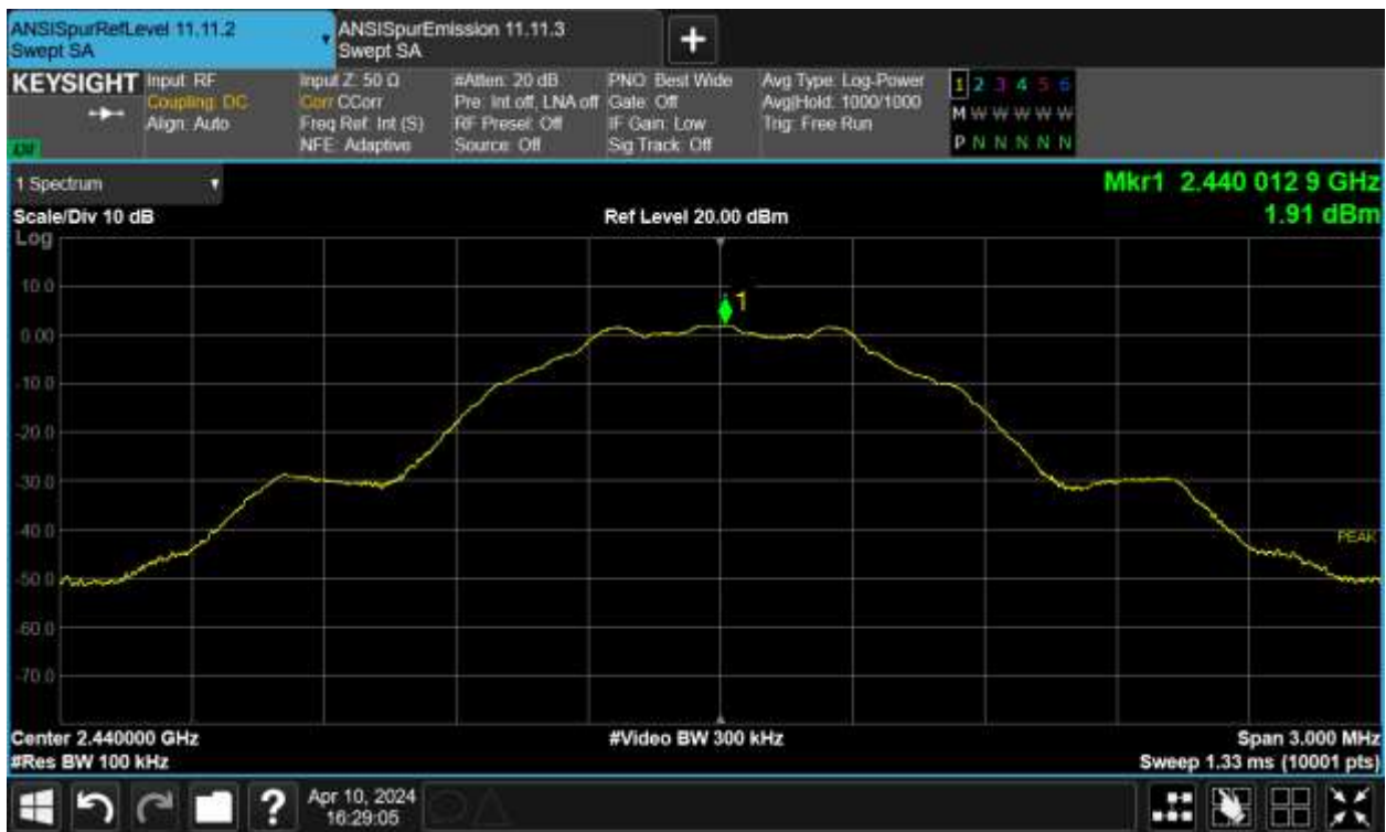
Figure TR27.2: Reference level measurement for Bluetooth BLE 1 Mbps at 2440 MHz
