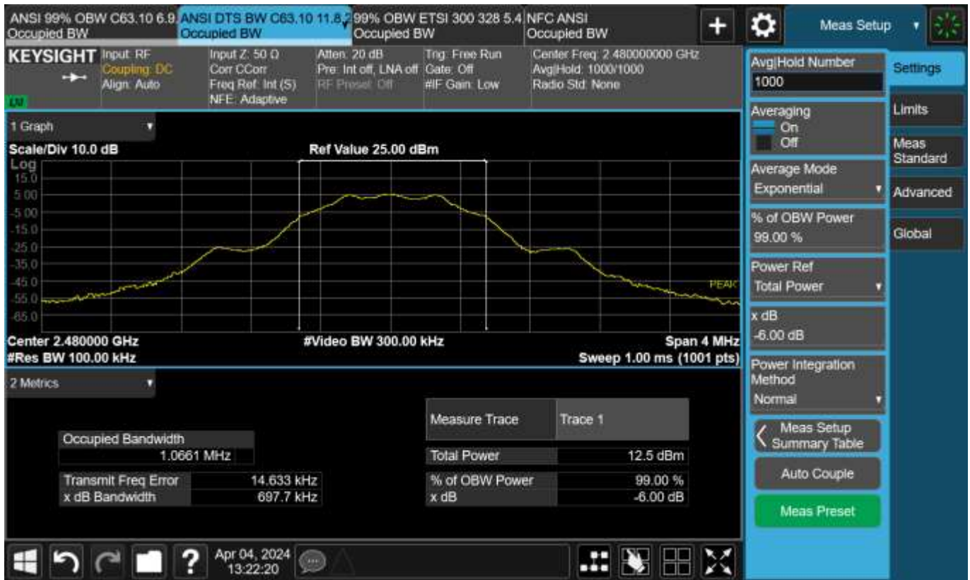
Figure TR06.3: Bandwidth data for BLE at high channel (2480 MHz)
