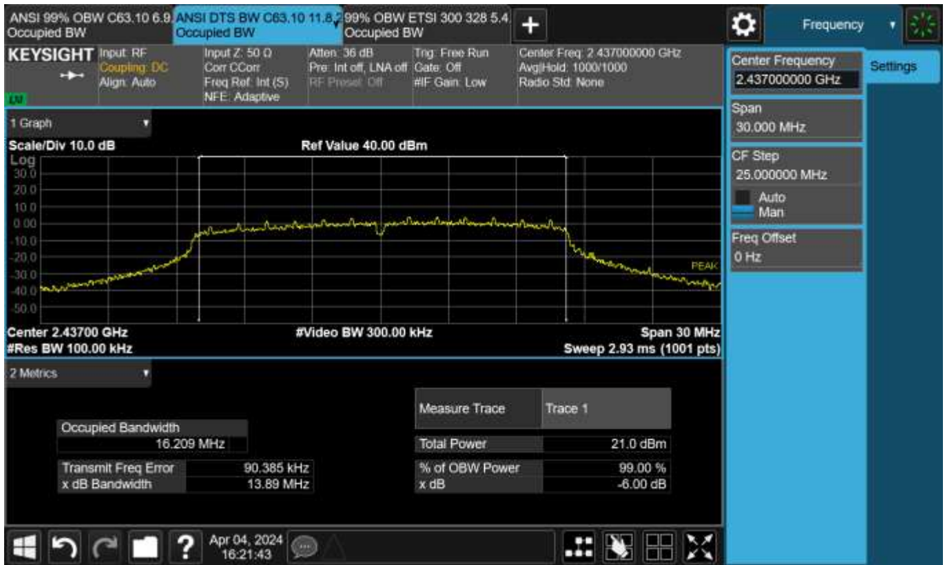
Figure TR06.5: Bandwidth data for 802.11g 9 Mbps at channel 6
