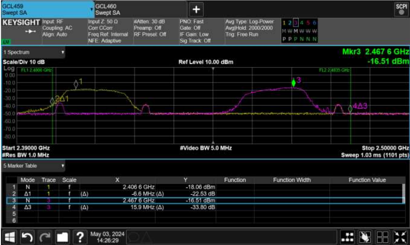
Figure TR44.1: Spectral plot for 60 °C and 5 V test condition
