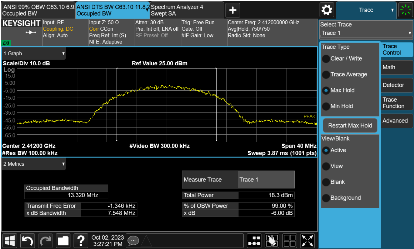
Figure TR08.2: Bandwidth data for 802.11b 11 Mbps at channel 1
