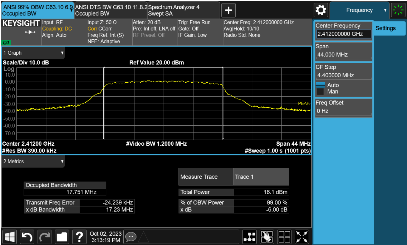
Figure TR10.5: Occupied bandwidth data for 802.11n MCS1 20MHz at channel 1
