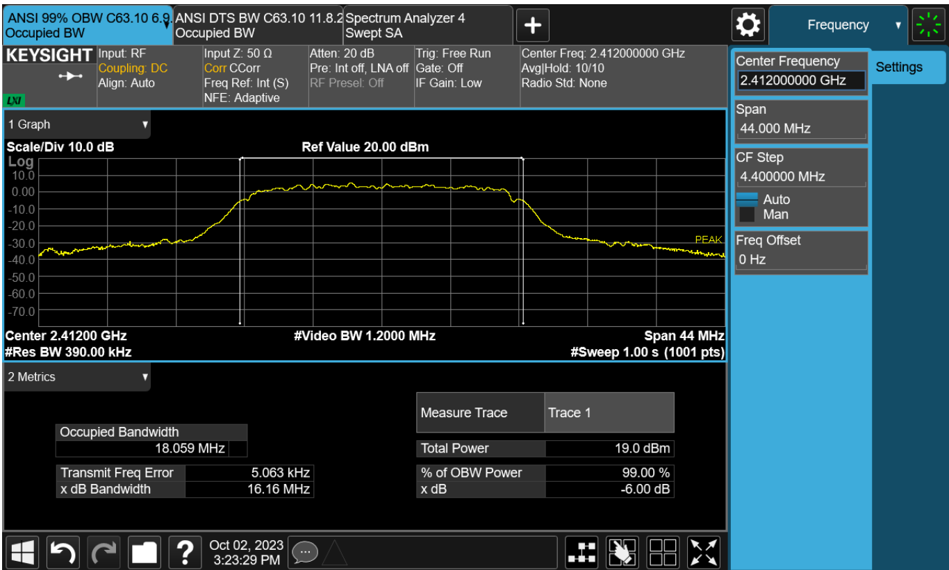
Figure TR10.4: Occupied bandwidth data for 802.11g 24 Mbps at channel 1
