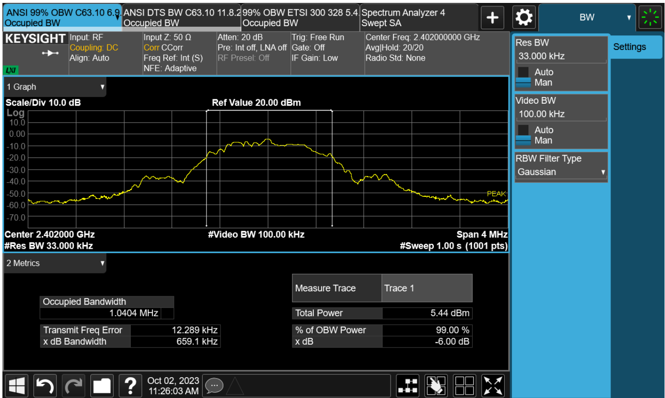
Figure TR10.2: Occupied bandwidth data for BLE at low channel (2402 MHz)
