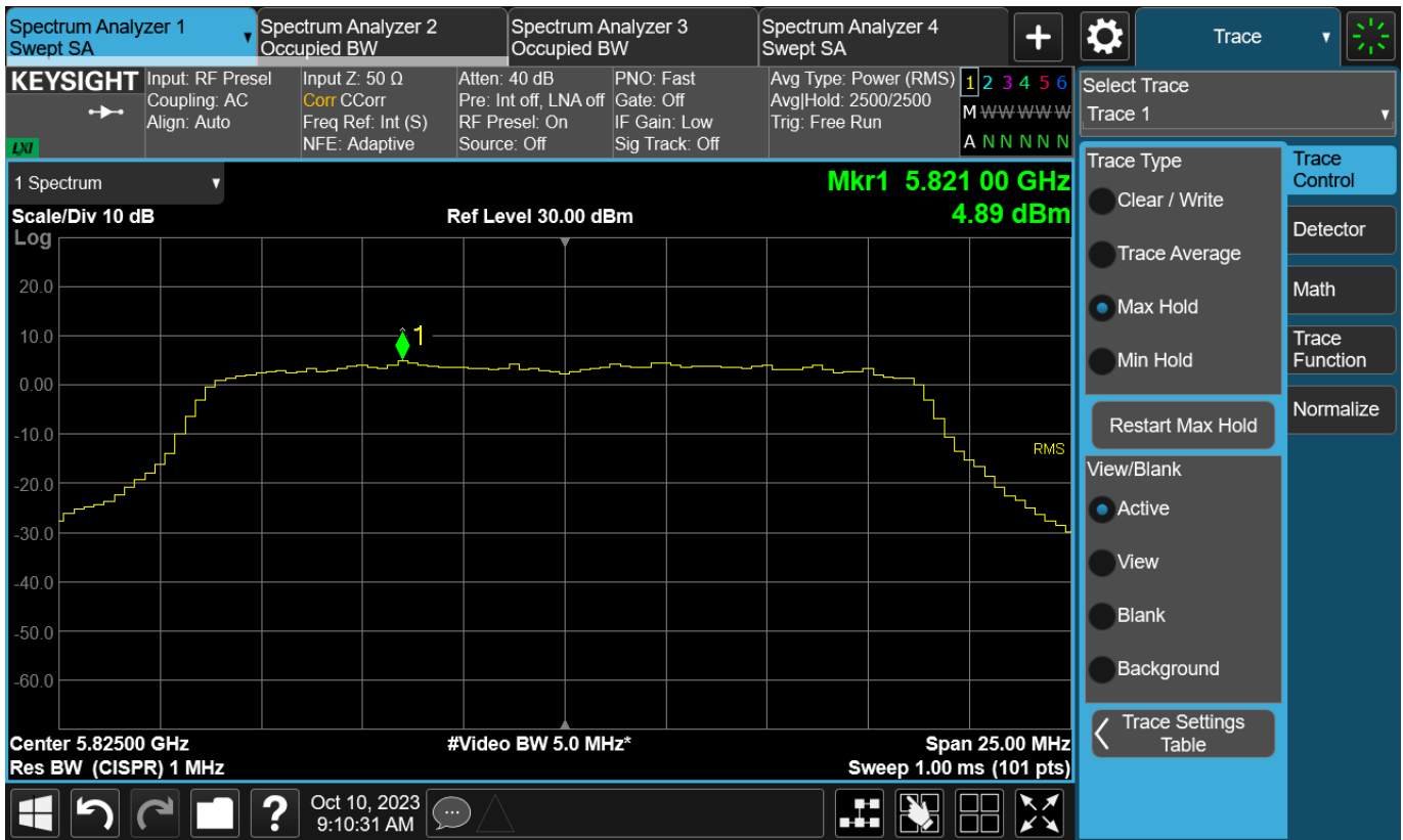
Figure TR17.6: Test data for 20 MHz MCS0 transmissions at 5825 MHz
