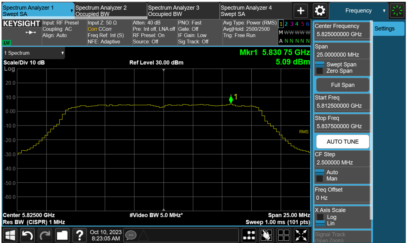
Figure TR17.4: Test data for A24 transmissions at 5825 MHz
