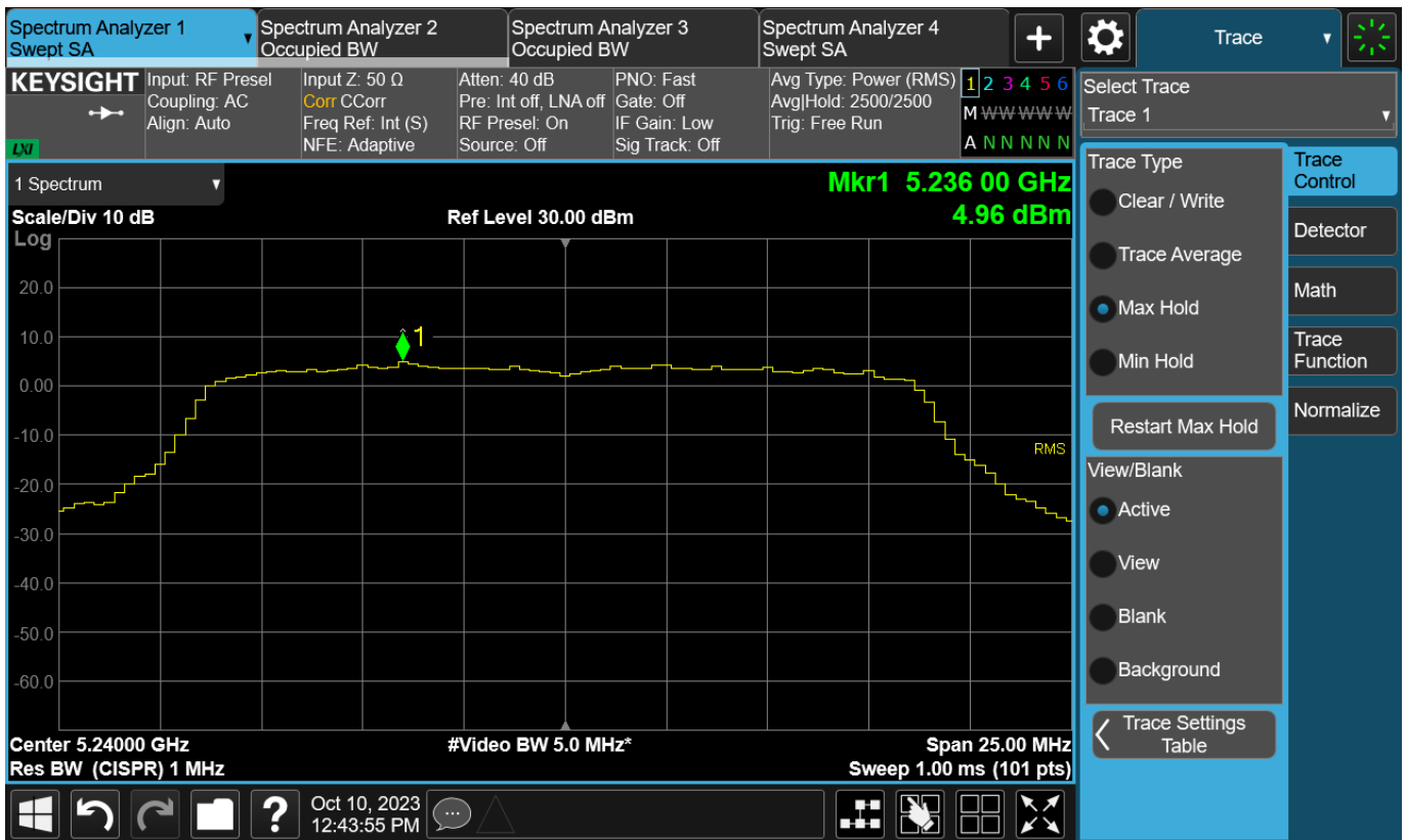
Figure TR17.5: Test data for 20 MHz MCS0 transmissions at 5240 MHz
