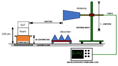
Figure 3 - Radiated Emissions Test Setup, >1GHz
