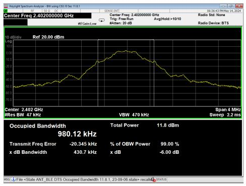
05 Occupied Bandwidth, Low Channel, GFSK
