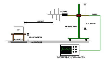
Figure 2 - Radiated Emissions Test Setup
