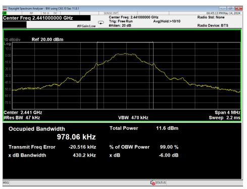
06 Occupied Bandwidth, Mid Channel, GFSK
