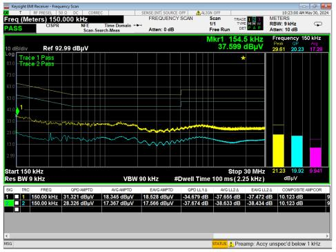
Figure 7 - Conducted Emissions Plot, Neutral, TX, 120VAC/60Hz
