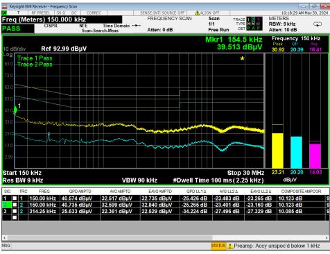
Figure 8 - Conducted Emissions Plot, Line, IDLE, 120VAC/60Hz
