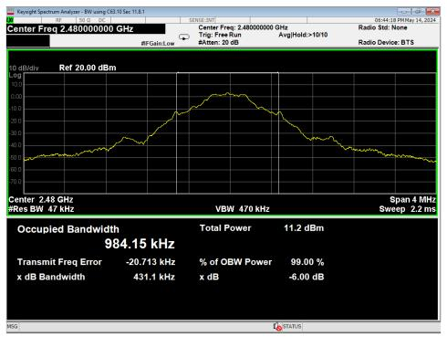
07 Occupied Bandwidth, High Channel, GFSK
