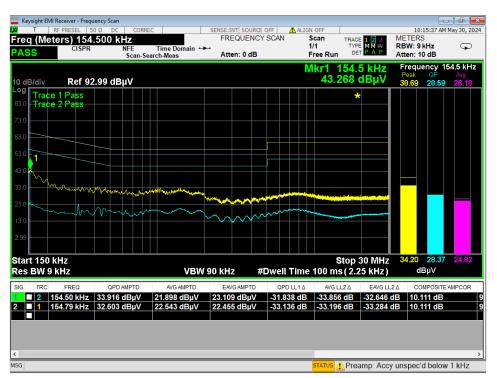
Figure 9 - Conducted Emissions Plot, Neutral, IDLE, 120VAC/60Hz
