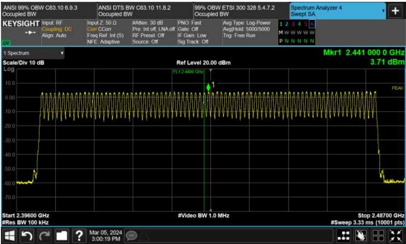
Figure TR32.1: Spectral data, Bluetooth Basic Rate transmission, showing channels used.
