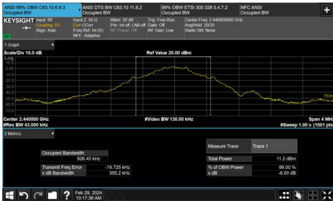
Figure TR09.2: Bandwidth data for Bluetooth at 2440 MHz
