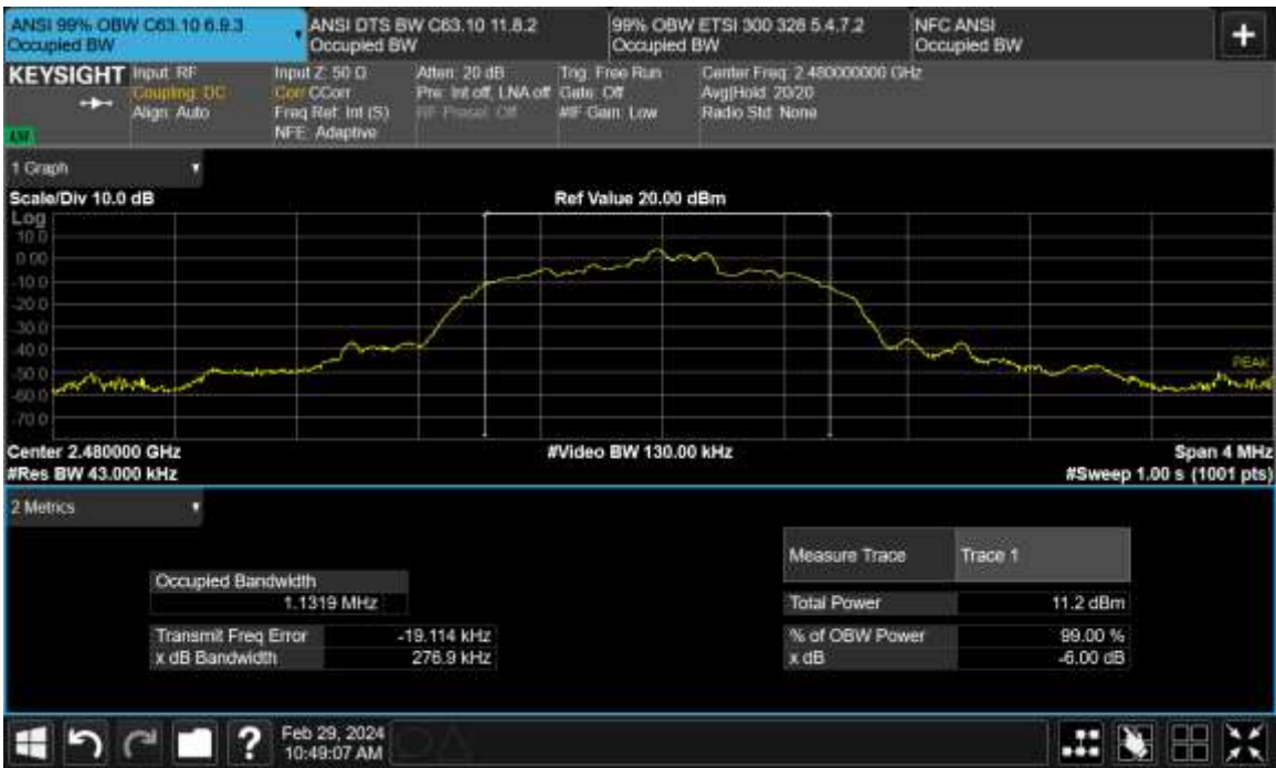
Figure TR09.4: Bandwidth data for Bluetooth EDR3 at 2480 MHz
