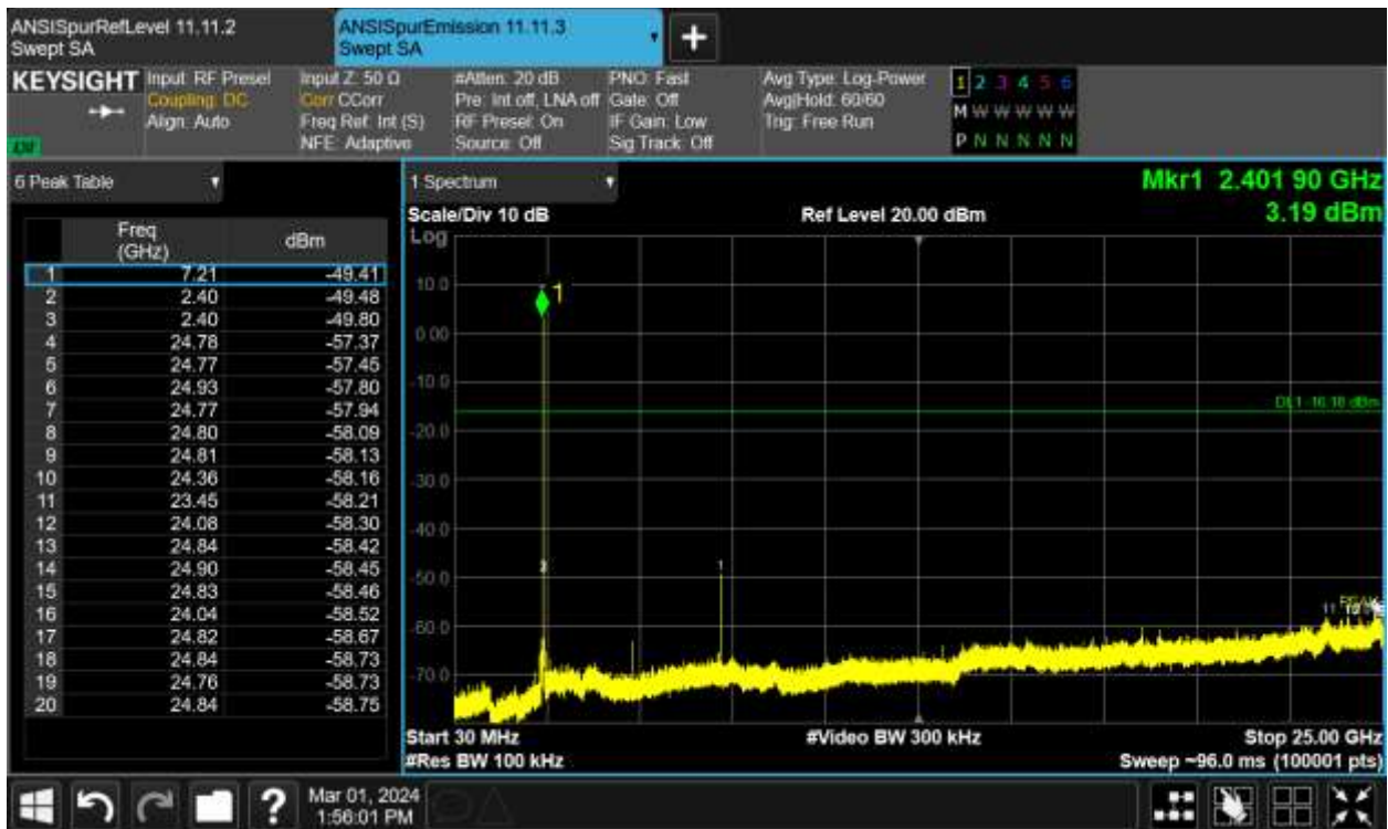
Figure TR36.3: Spectral data for Bluetooth Basic Rate at 2402 MHz
