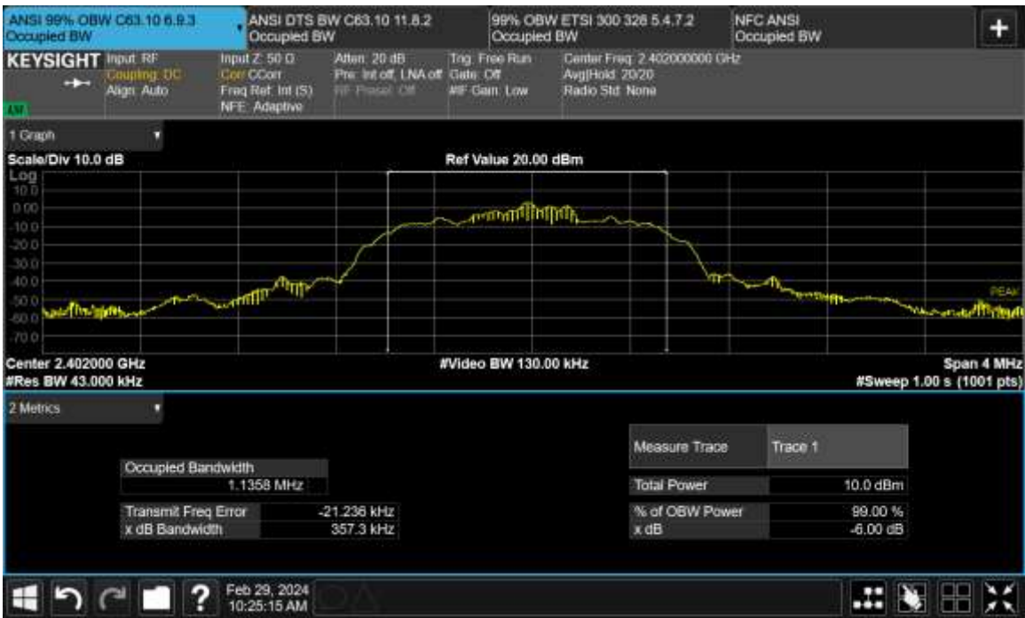
Figure TR09.3: Bandwidth data for Bluetooth ERD2 at 2402 MHz
