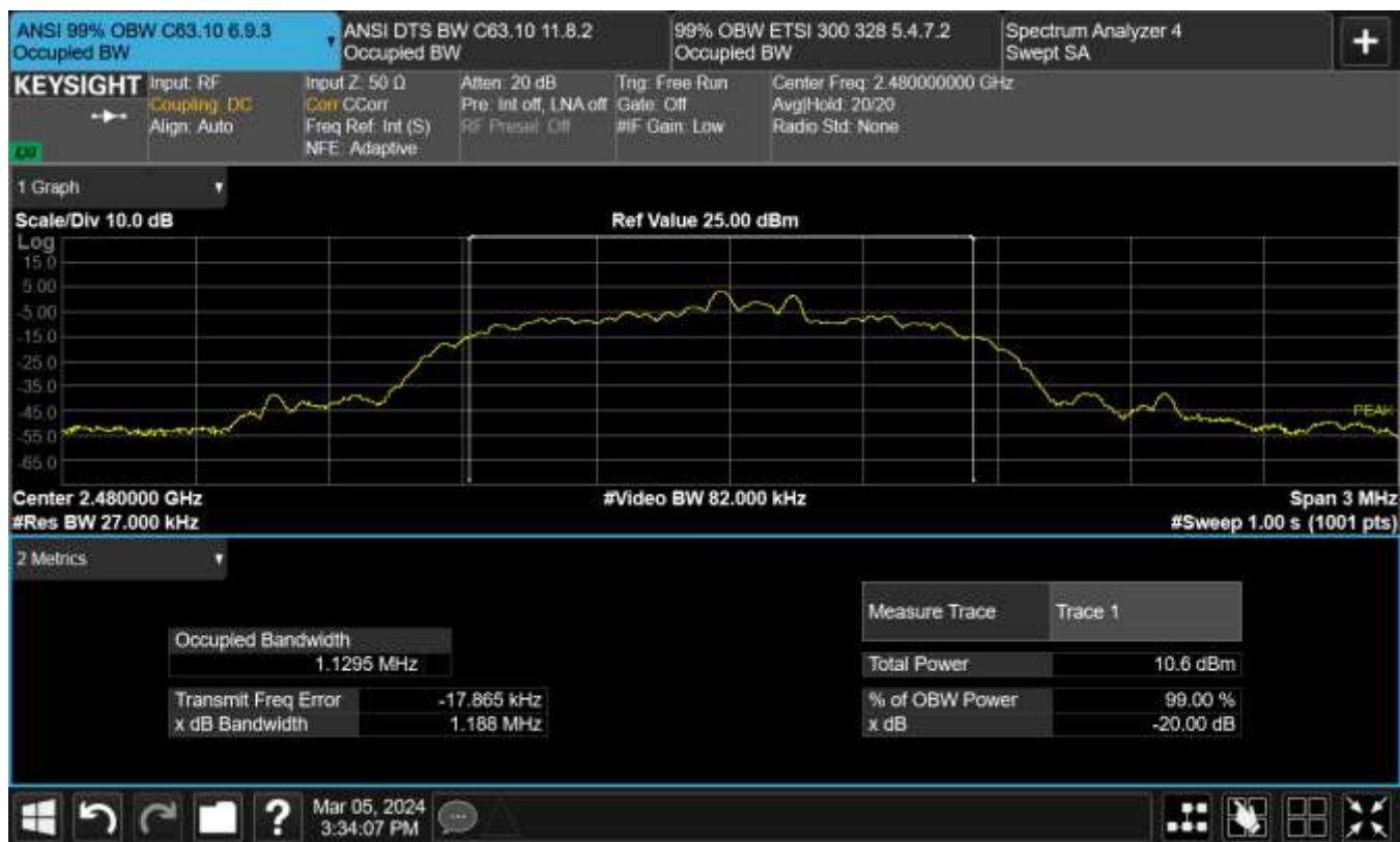
Figure TR32.2: Spectral data for Bluetooth EDR3 modulation at 2480 MHz
