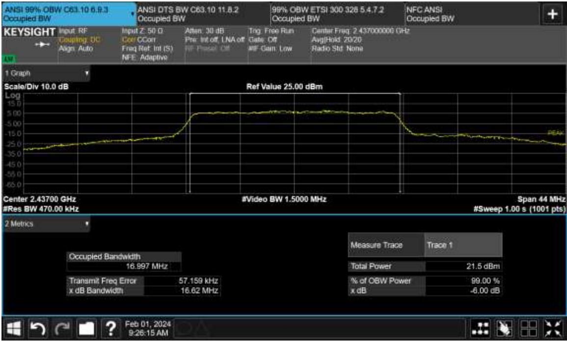
Figure TR10.6: Bandwidth data for G36 Modulation on Channel 6 (2440 MHz)
