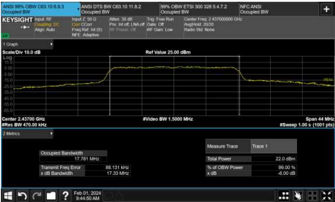
Figure TR10.7: Bandwidth data for NMCS5 Modulation on Channel 6 (2440 MHz)
