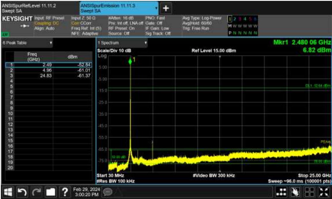
Figure TR27.3 Spectral data for Bluetooth BR at 2480 MHz
