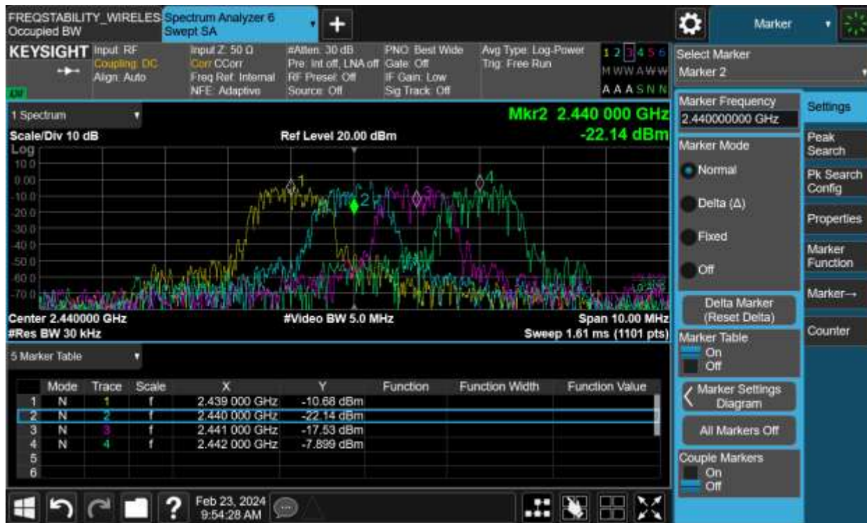
Figure TR50.2: Spectral data, Bluetooth transmissions, showing four specific channels used
