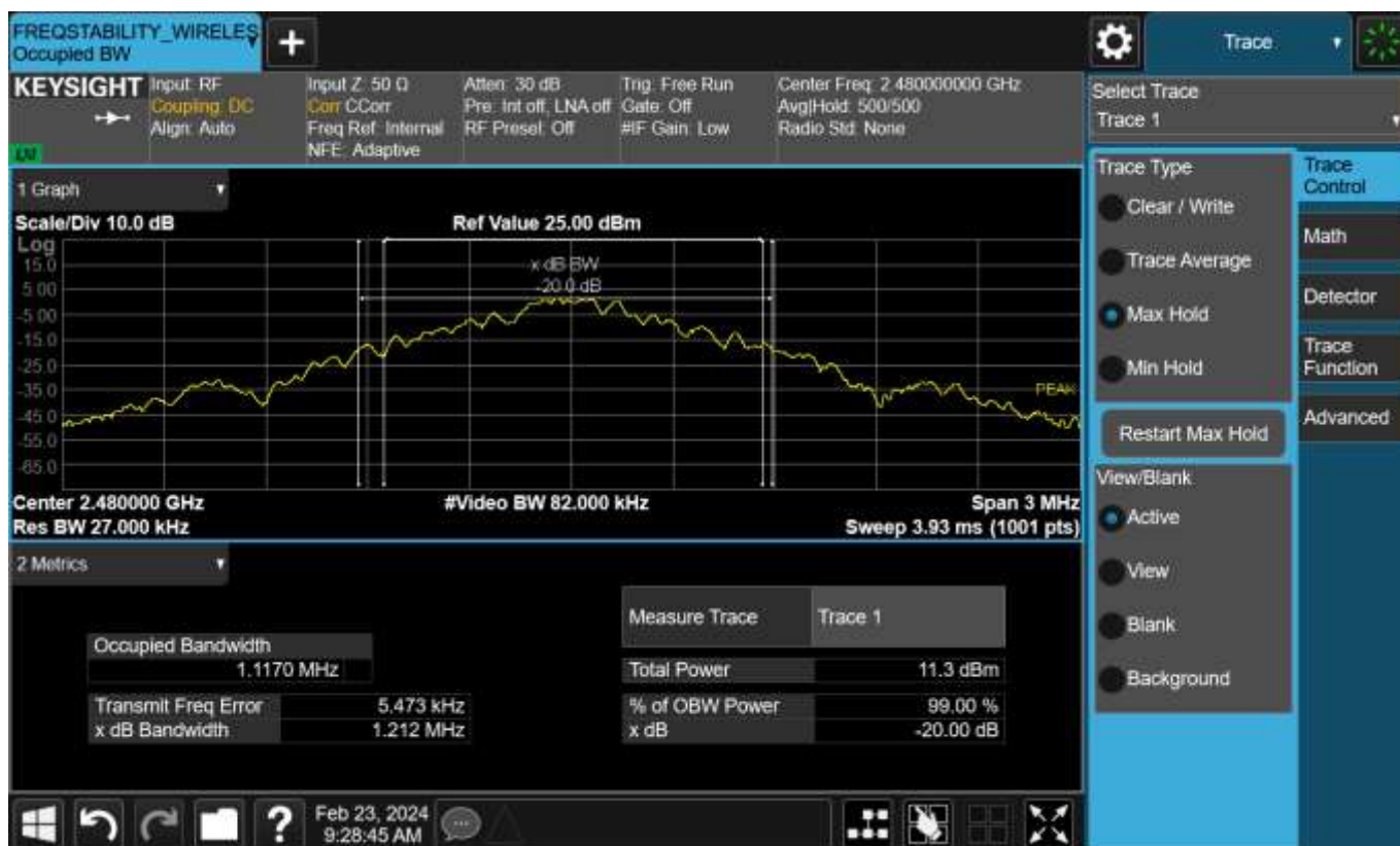
Figure TR50.3: Spectral data for EDR3 modulation at 2480 MHz
