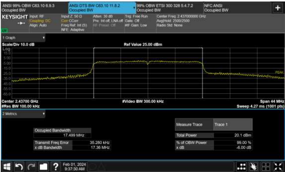
Figure TR07.6: Bandwidth data for 802.11n MCS2 at channel 6
