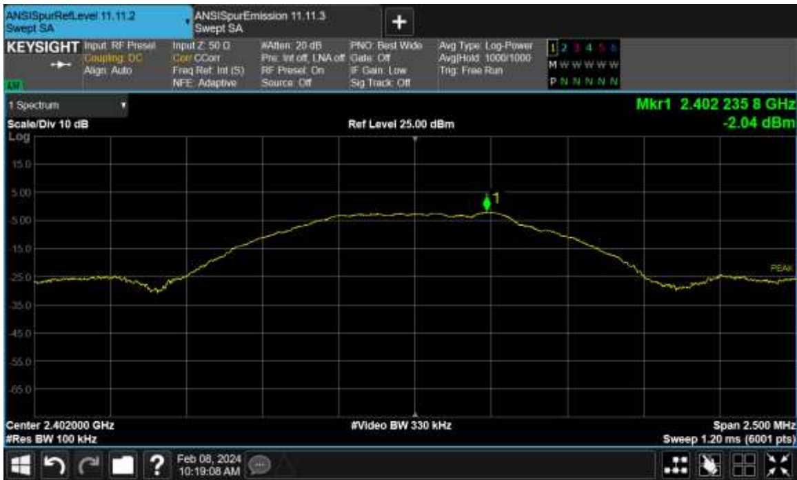
Figure TR28.2: Reference level measurement for Bluetooth BLE 1 Mbps at 2402 MHz
