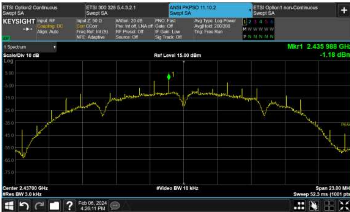
Figure TR20.4: Test data for WiFi mode B1 Mbps, Ch6
