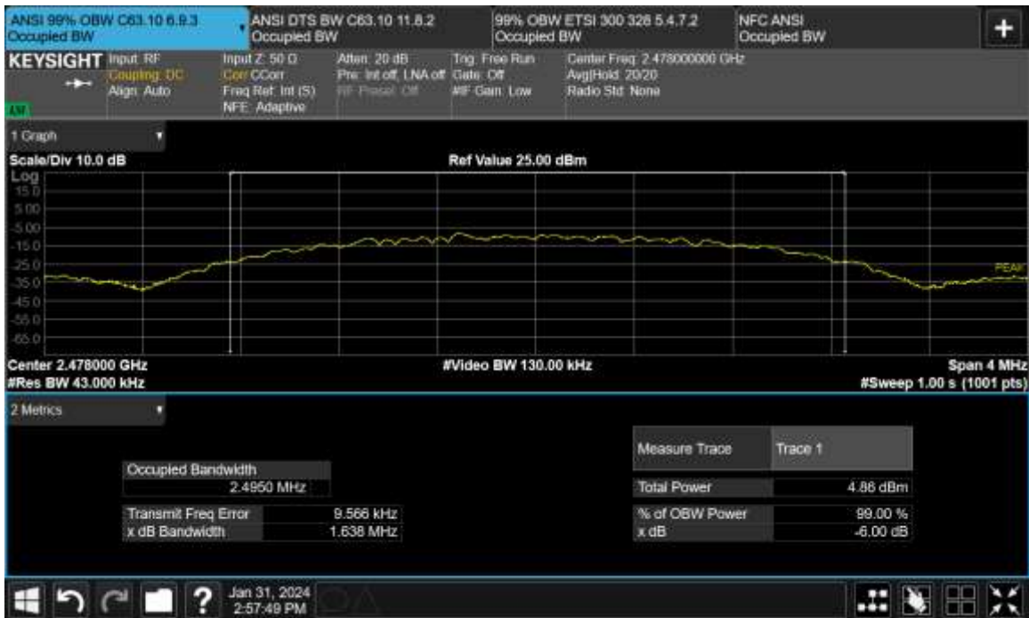
Figure TR10.3: Bandwidth data for BLE 2 Mbps at 2478 MHz
