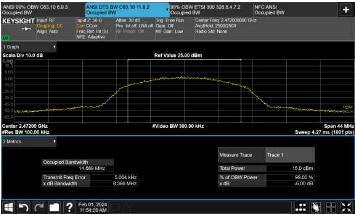
Figure TR07.4: Bandwidth data for 802.11b 5.5 Mbps at channel 13
