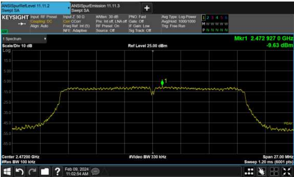
Figure TR28.10: Reference level measurement for IEEE 802.11 N MCS0 on Ch.13
