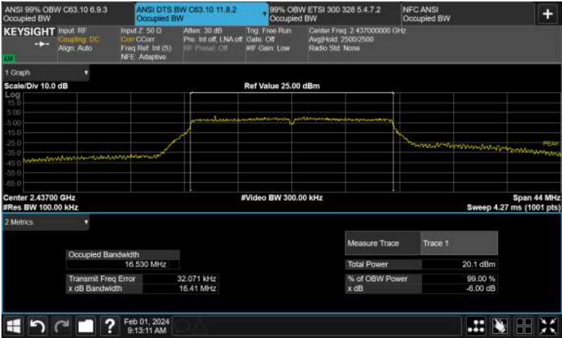
Figure TR07.5: Bandwidth data for 802.11g 6 Mbps at channel 6
