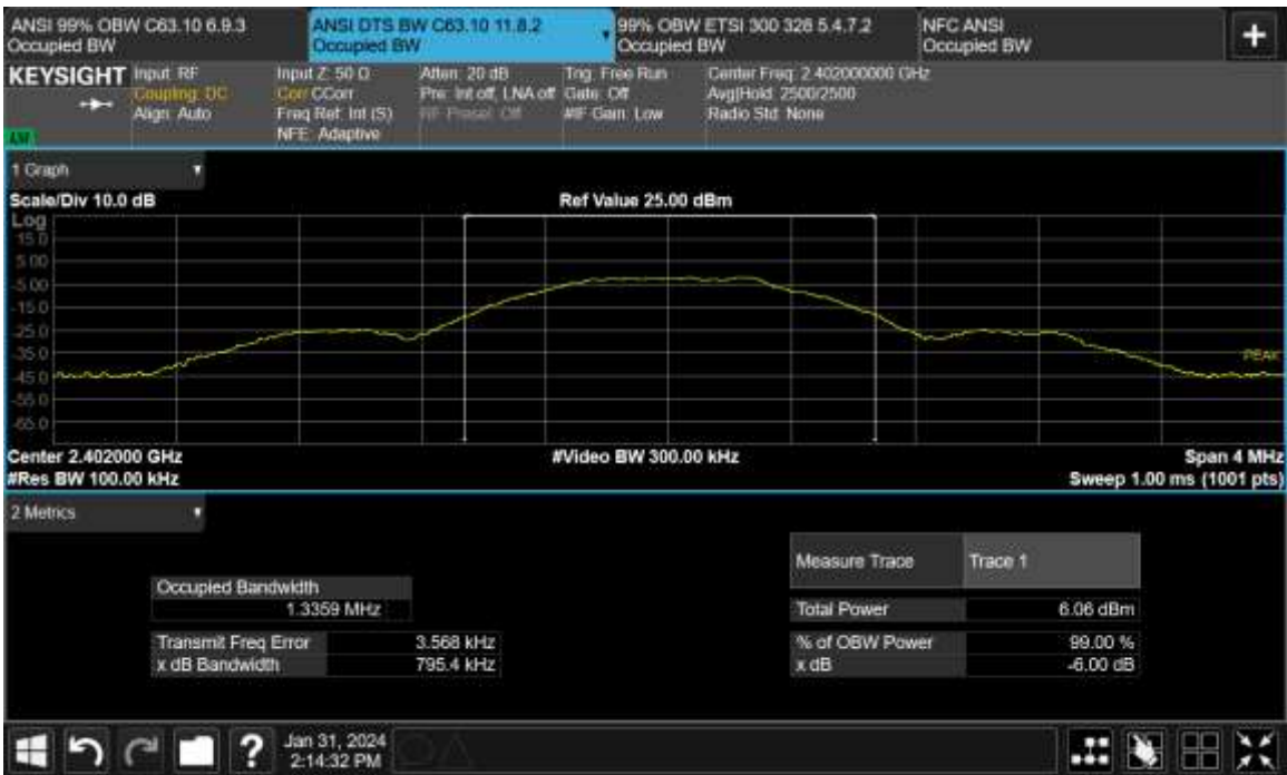
Figure TR07.2: Bandwidth data for BLE 1 at low channel (2402 MHz)
