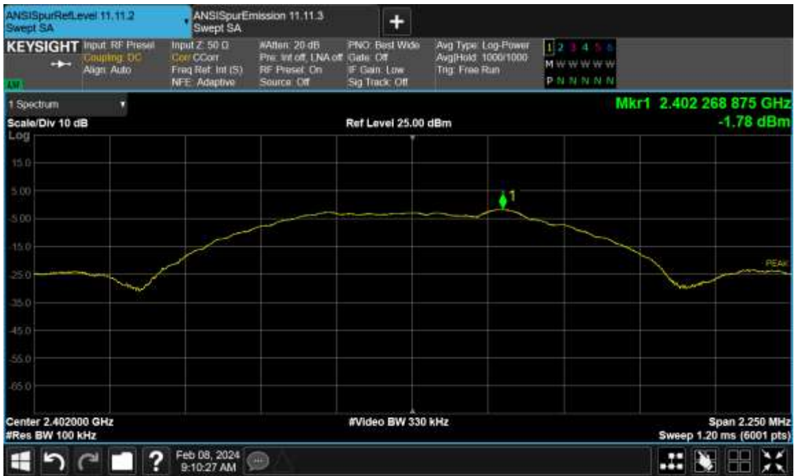
Figure TR28.4: Reference level measurement for ANT at 2402 MHz
