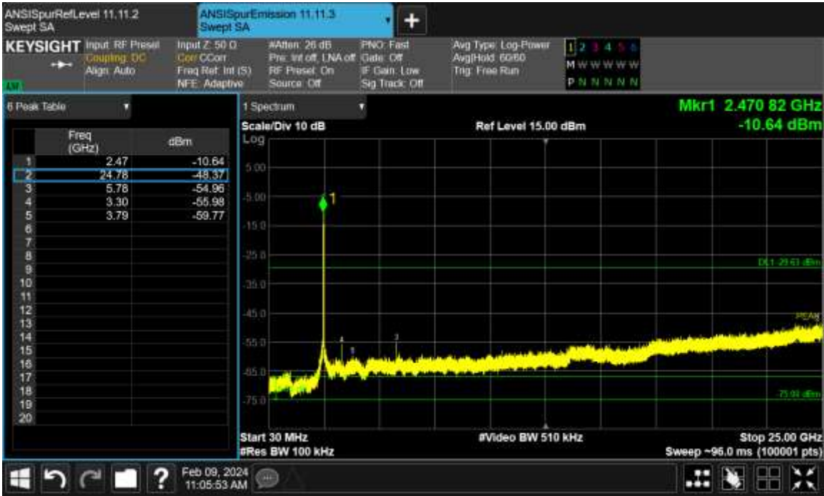
Figure TR28.11 Spectral data for IEEE 802.11 N MCS0 on Ch.13
