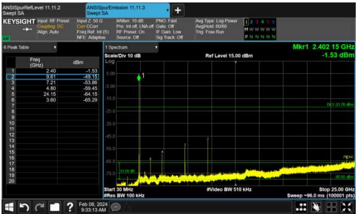
Figure TR28.5 Spectral data for ANT at 2402 MHz
