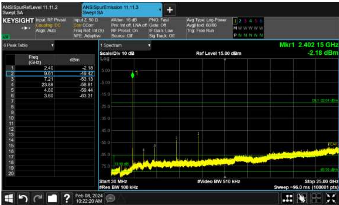
Figure TR28.3 Spectral data for Bluetooth BLE 1 Mbps at 2402 MHz
