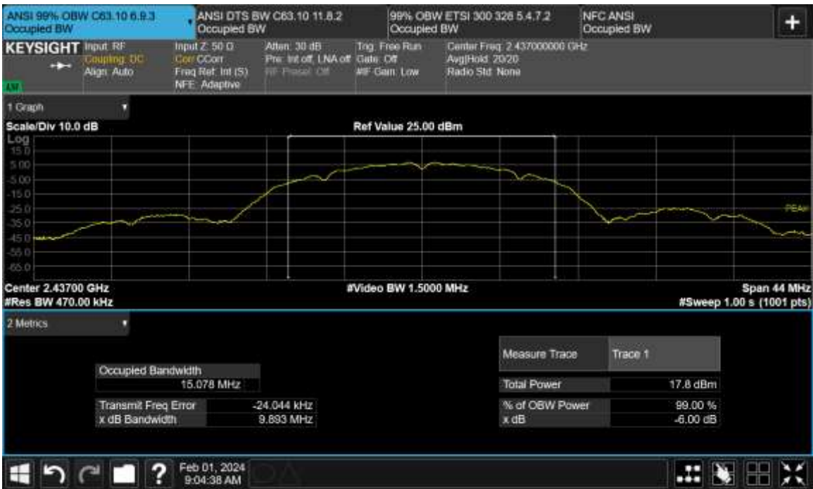
Figure TR10.5: Bandwidth data for B2 Modulation on Channel 6 (2440 MHz)
