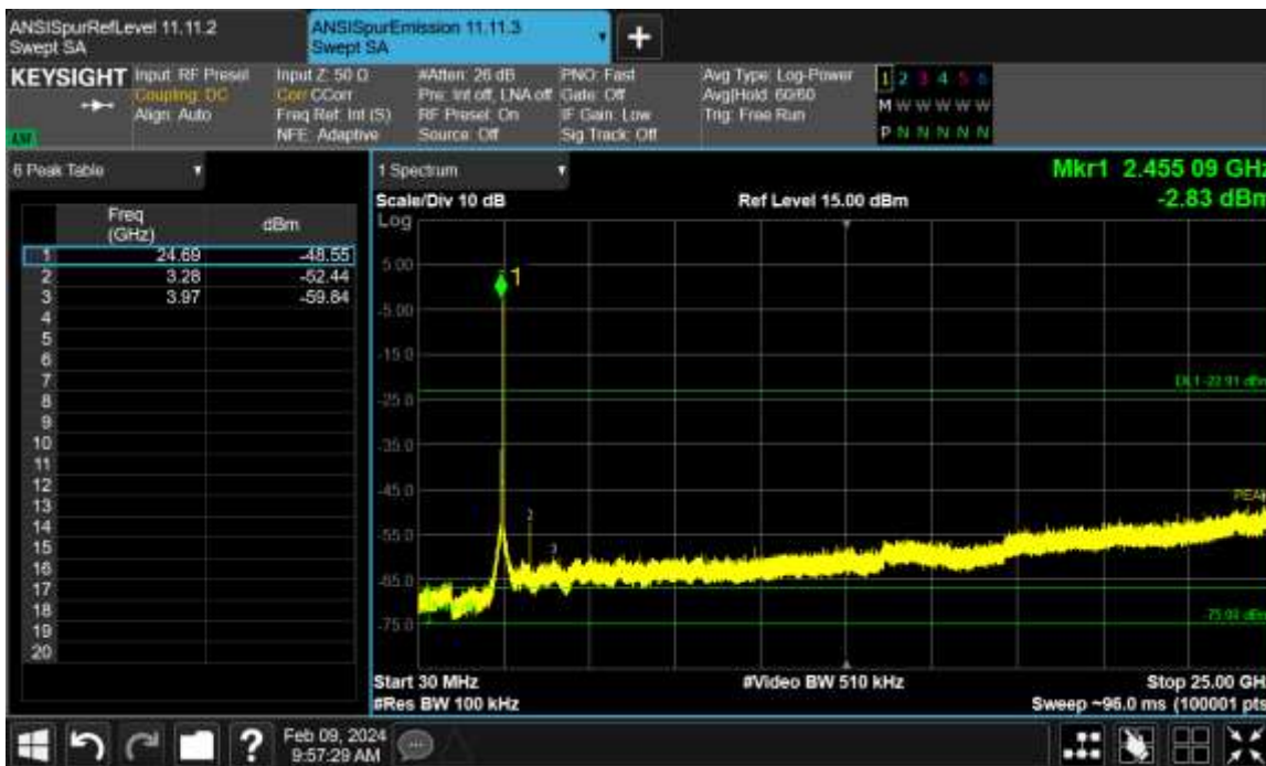
Figure TR28.9 Spectral data for IEEE 802.11 G 24 Mbps on Ch.11
