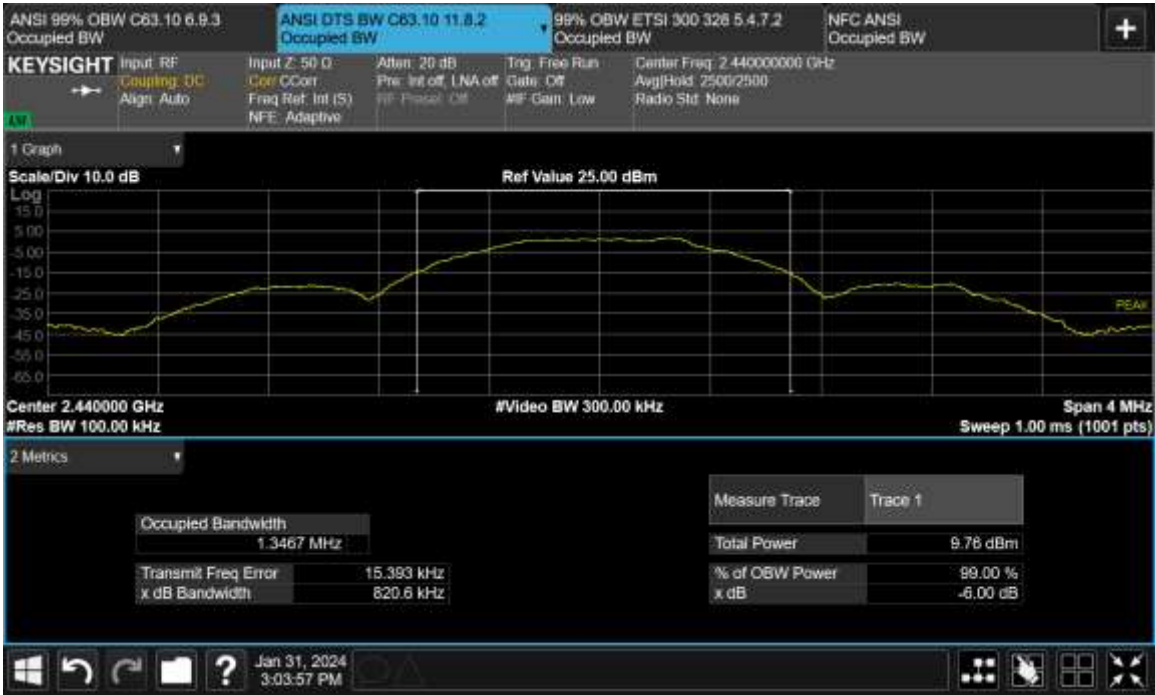
Figure TR07.3: Bandwidth data for ANT at mid channel (2440 MHz)
