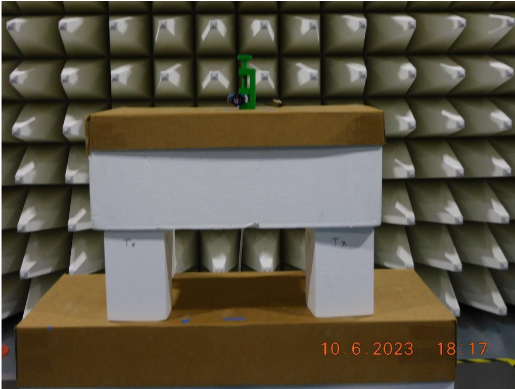
Figure RE09.2: EUT test setup, front view
