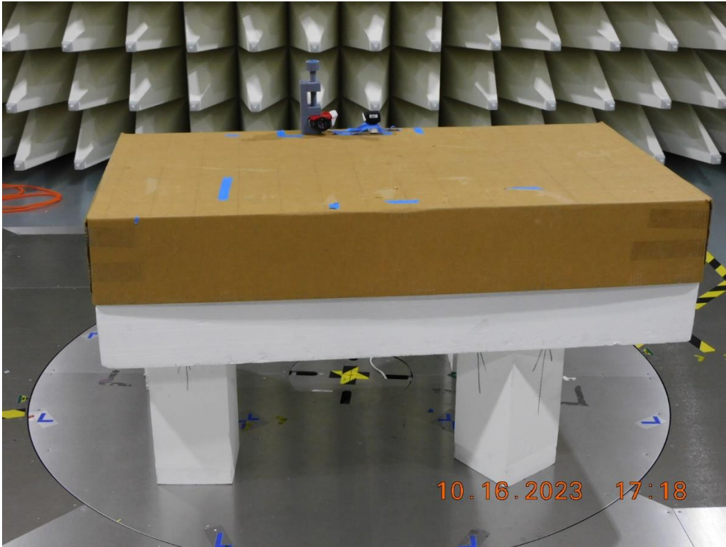
Figure RE07.4: EUT test setup, front view (X orientation)
