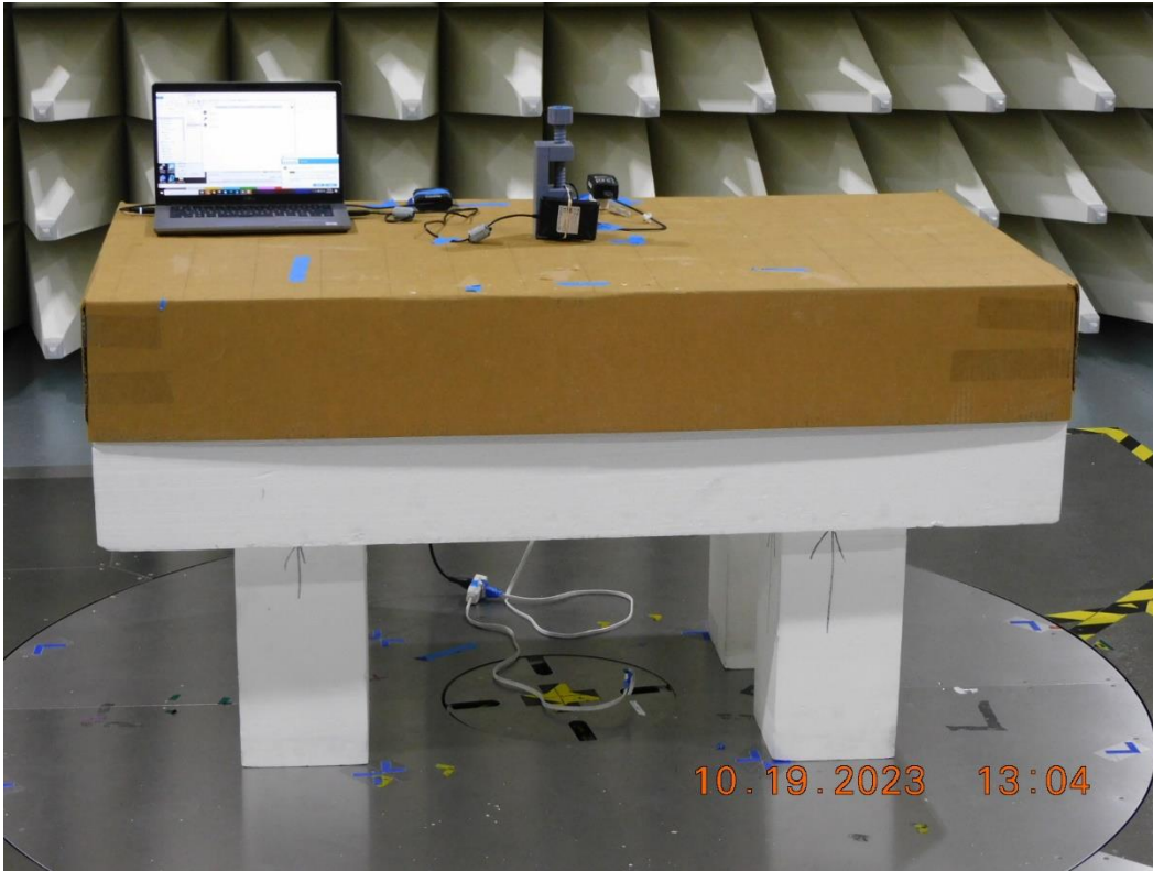
Figure RE13.2: EUT test setup, front view (X orientation)
