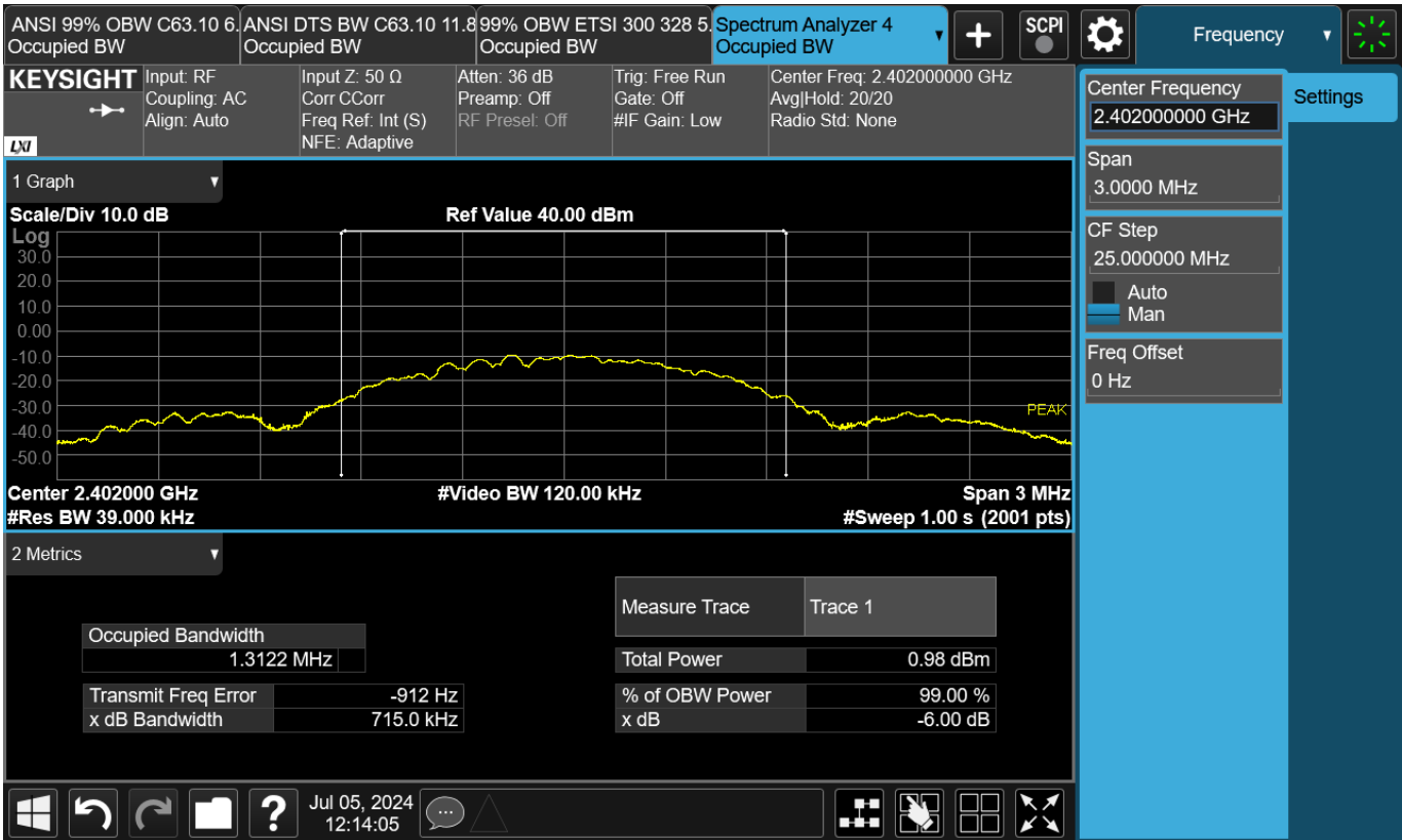
Figure TR10.2: Occupied bandwidth data for BLE, 1 Mbps at low channel (2402 MHz)
