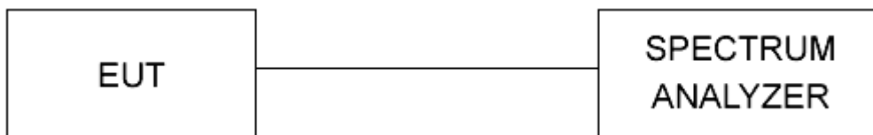
Figure 1 - Bandwidth Measurements Test Setup
