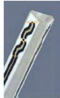
Figure 2.3 Probe Thick-Film Technique
