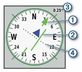
The course pointer ① indicates your relationship to the course line leading to the destination. The course deviation indicator (CDI) ② provides the indication of drift (right or left) from the course. The scale ③ refers to the distance between dots ④ on the course deviation indicator, which tell you how far off course you are.
