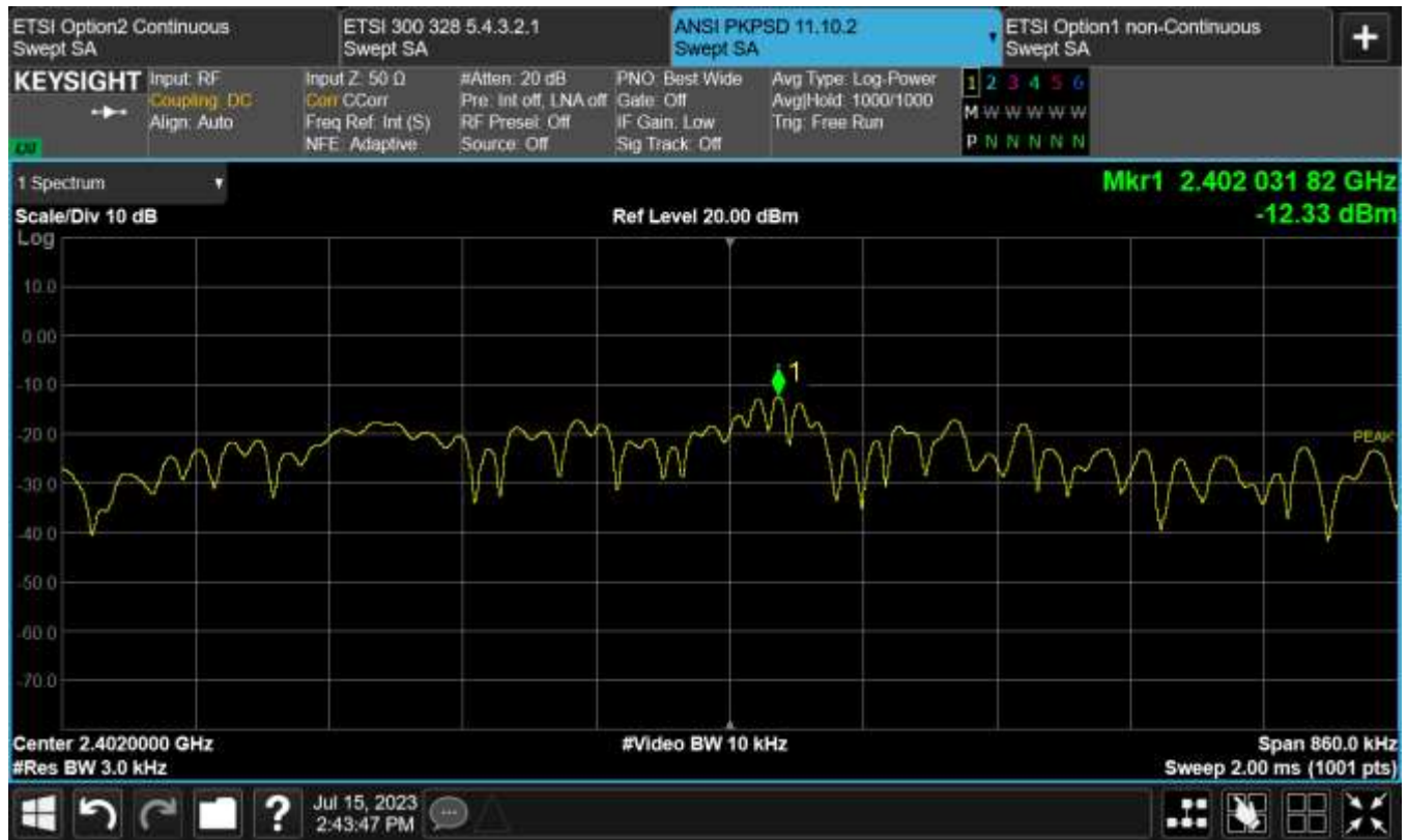
Figure TR03a.2: Test data for BLE at 1 Mb/s, 2402 MHz
