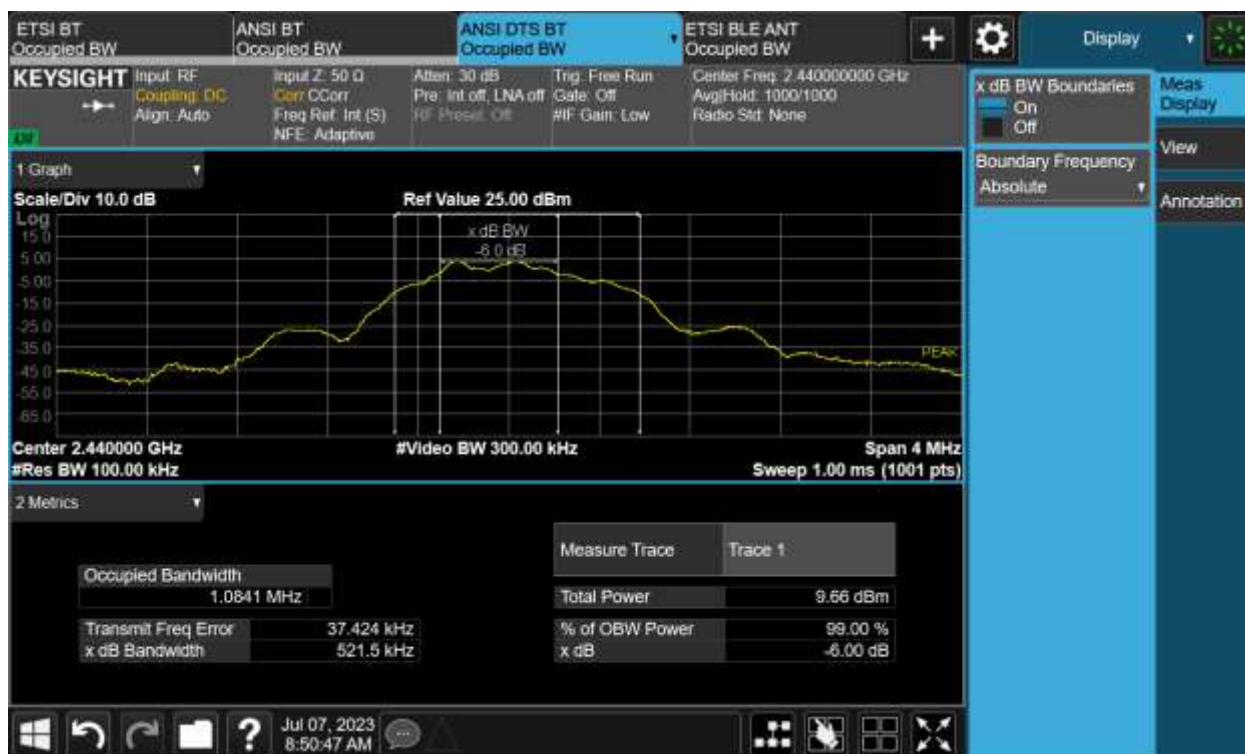
Figure TR02a.2: Bandwidth data for BLE at mid channel (2440 MHz)
