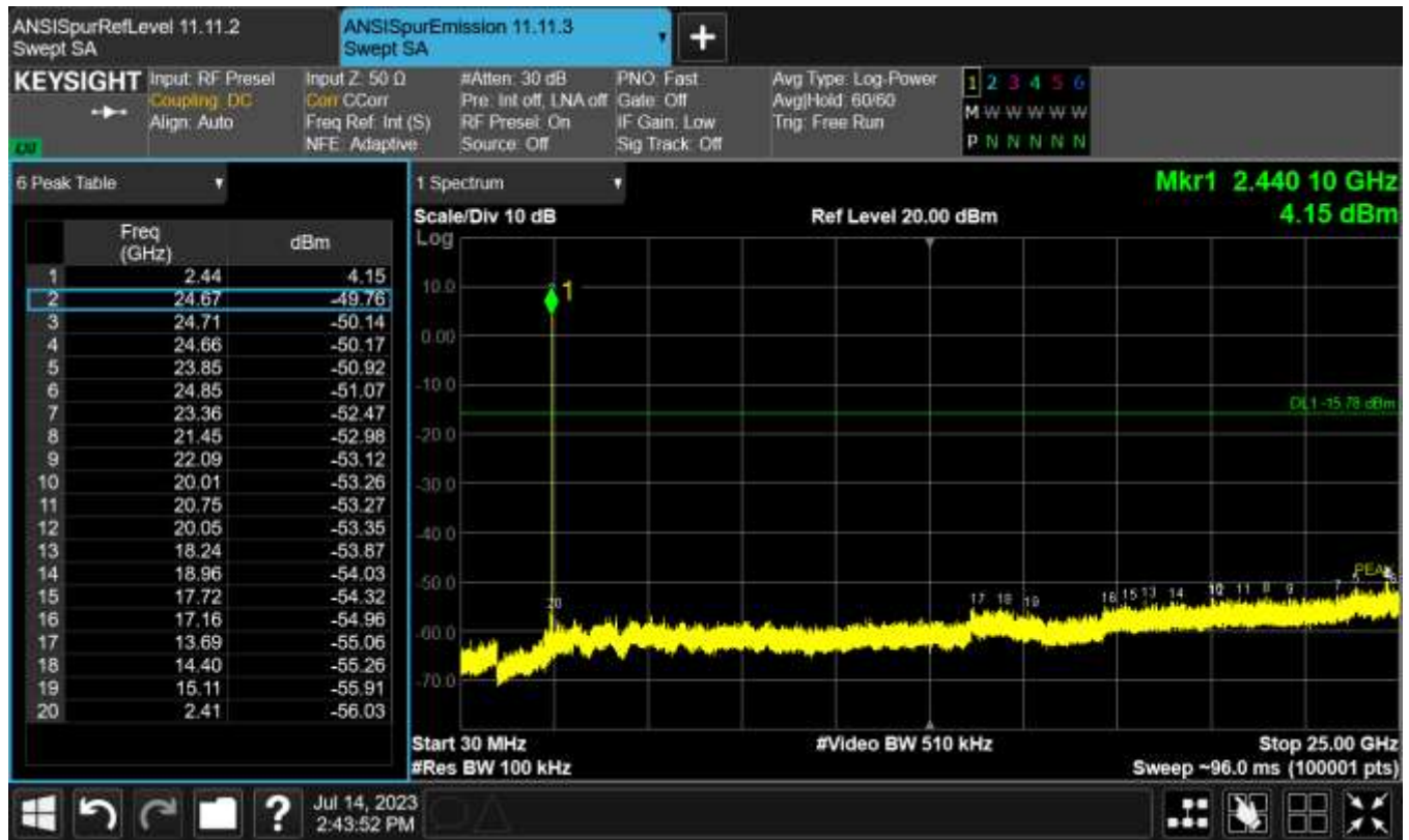
Figure TR05.2: Spectral data for Bluetooth BLE 1 Mbps at 2440 MHz
