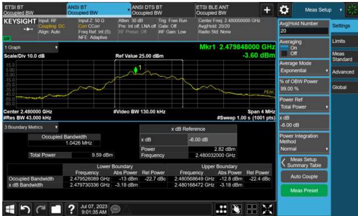
Figure TR02b.2: Bandwidth data for BLE at high channel (2480 MHz)
