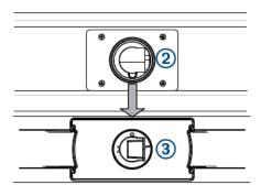
3 Secure the antenna to the pedestal using the included hex bolts (4) and spring washers (5).
