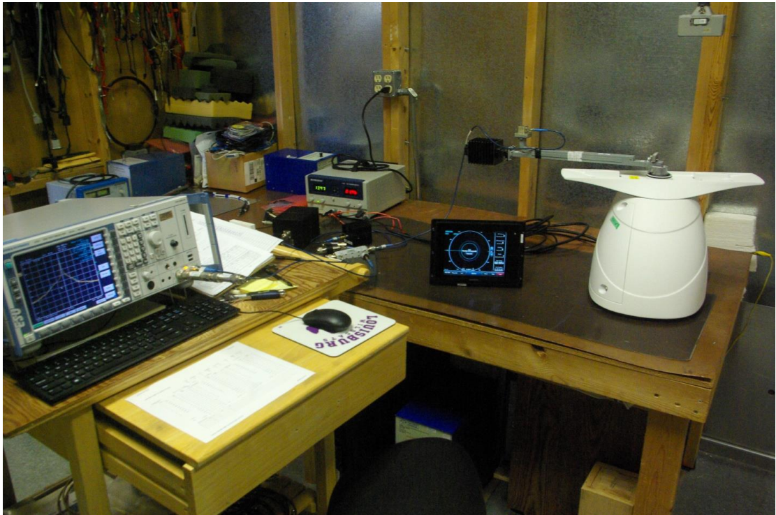
Antenna Port Conducted Emissions Test Setup
