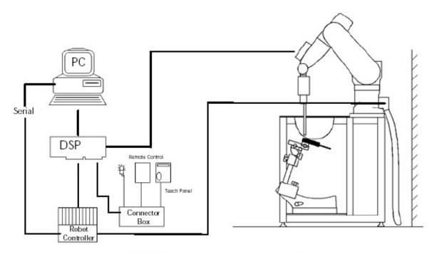
Figure 2.1 SAR Measurement System Setup
