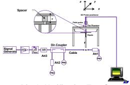
**Figure 7.1 Dipole Verification Test Setup**
