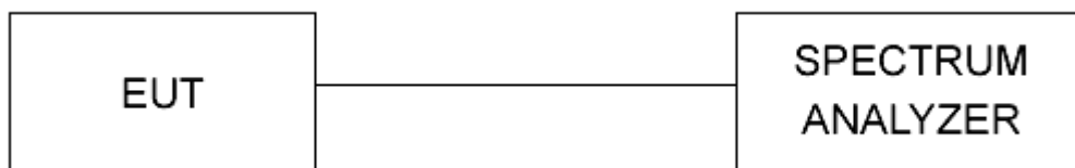
Figure 1 - Bandwidth Measurements Test Setup
