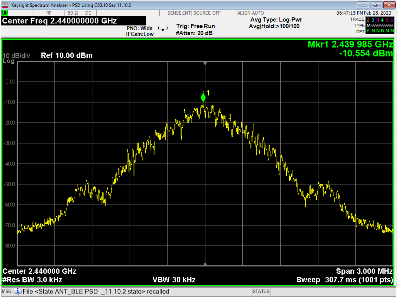
08 PSD, Mid Channel, GFSK
