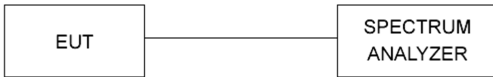
Figure 1 - Bandwidth Measurements Test Setup
