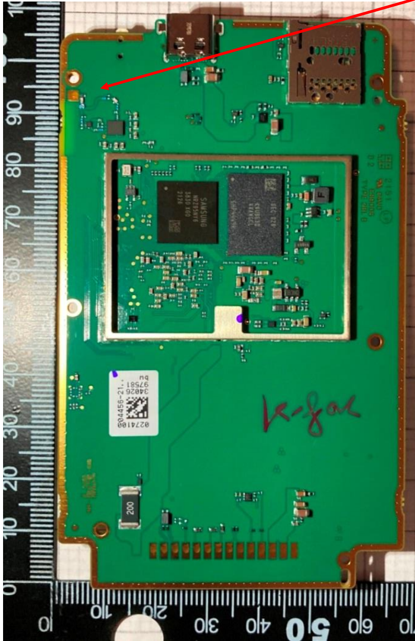
Bottom Shield removed and Antenna Connection point
