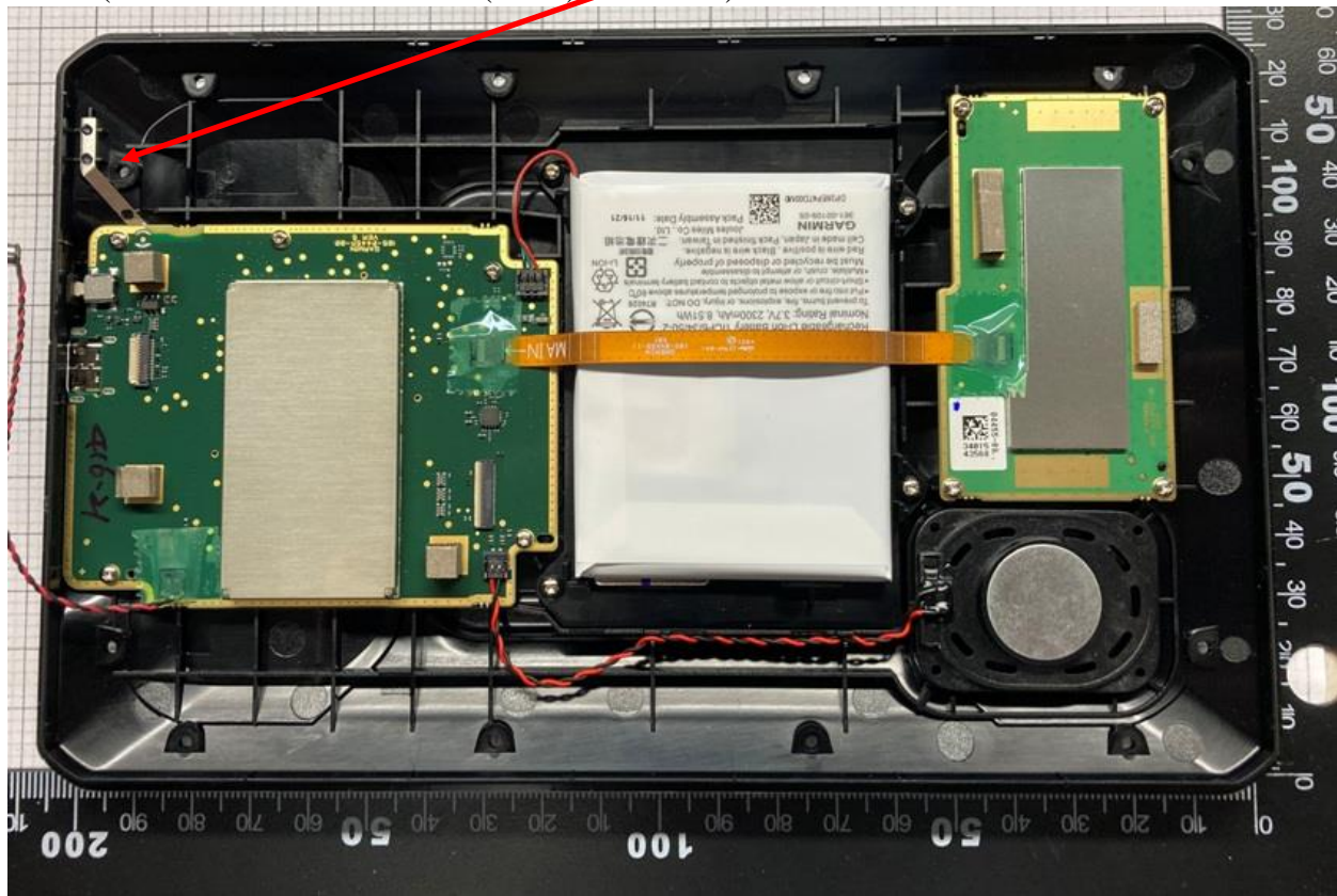
Internal photographs of equipment under test Inside (Planar Inverted F Antenna (PIFA) locations )
