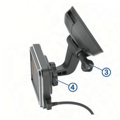
4 Tighten the thumbscrew on the suction cup arm and the nut on the ball mount.
