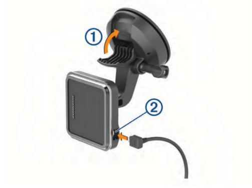
2 Plug the vehicle power cable into the port 2 on the mount.
