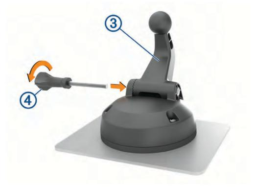
6 Insert the thumbscrew 4 into the mount, and tighten it to secure the ball mount arm.
