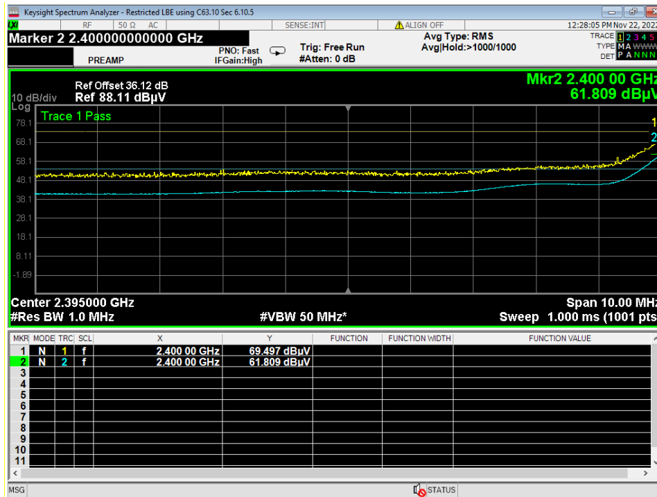
04 Lower Bandedge, Unrestricted, GFSK, 15.209 limits Disregard trace 2, duty cycle correction was added to peak level
